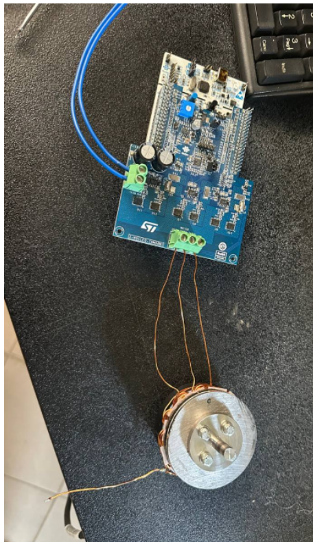
(a) Connection to the ST inverter/control board.
