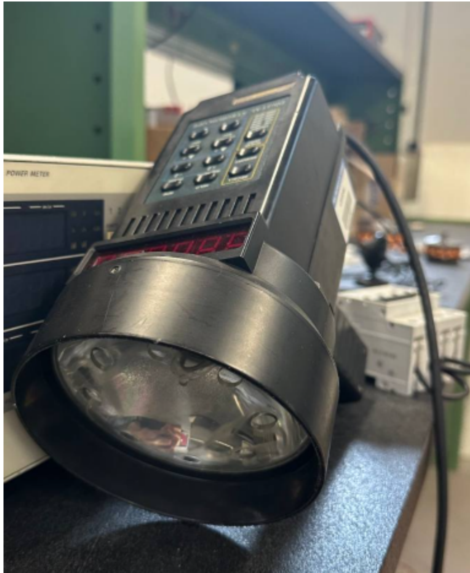
Figure 3.4: Manual speed-measurement instrument used as an additional reference during the laboratory activity.
