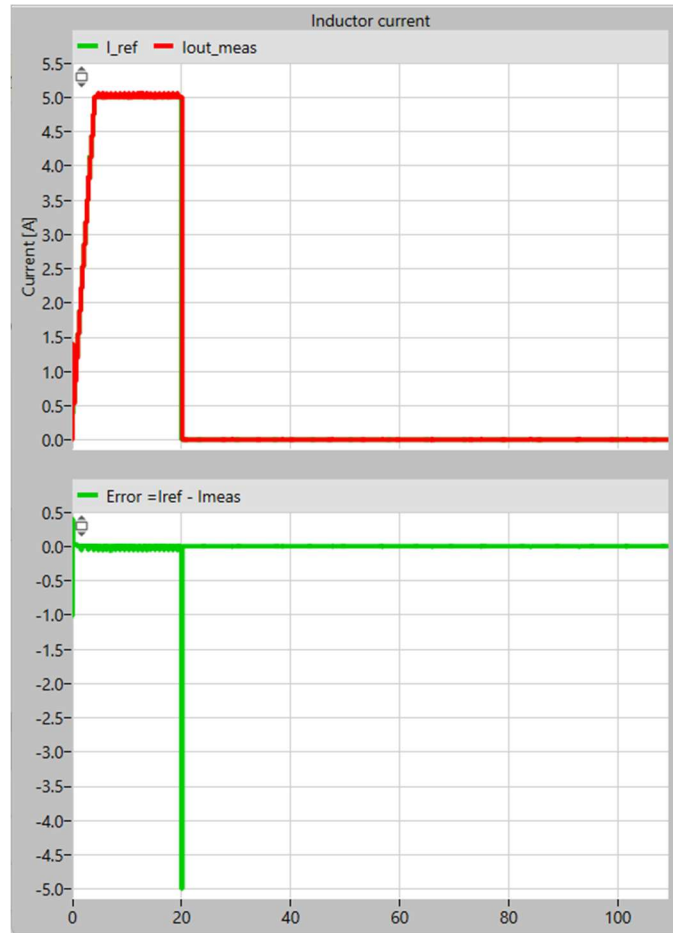
Figure 6.14 Inductor Current Tracking Performance During the Charging Process in Buck-Mode Operation
