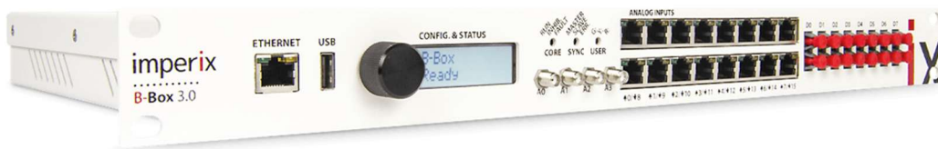
Figure 7.2. B-Box RCP controller used for real-time execution of the converter control algorithm
