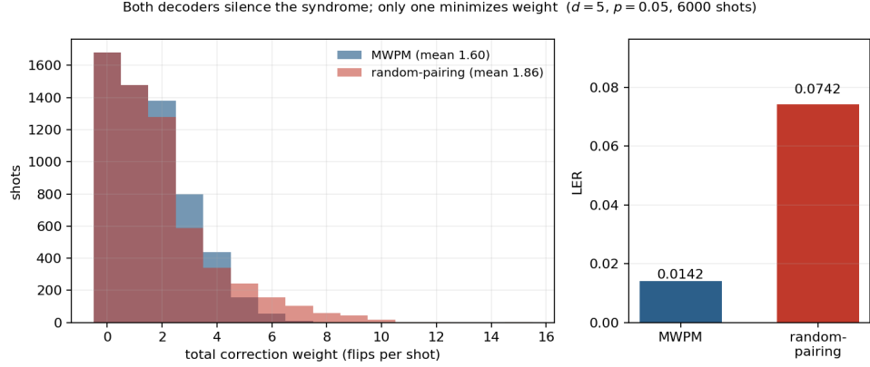
Figure 8.3: The cost of non-minimality: MWPM versus a random-pairing decoder that silences the same syndromes with heavier corrections ( d = 5, p = 0.05, 6000 shots, same error samples). A 16% average weight excess translates into a 5\times higher logical error rate: the extra weight means a higher probability of pairing defects along the wrong homology class
