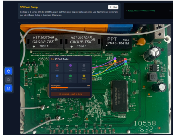
Figure 6.6: The SPI firmware dumper during a dump operation. Six colour-coded probes are connected to the flash chip. The progress bar shows the simulated read address advancing.
