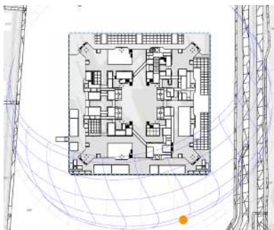
Figure 5.134: Winter solstice solar penetration at 12:00
