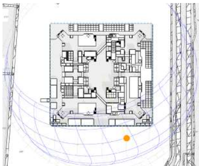
Figure 5.131: Autumnal equinox solar penetration at 12:00
