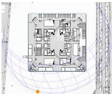
Figure 5.135: Winter solstice solar penetration at 15:00
