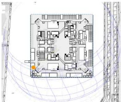
Figure 5.129: Summer solstice solar penetration at 15:00
