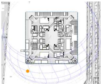
Figure 5.132: Autumnal equinox solar penetration at 15:00
