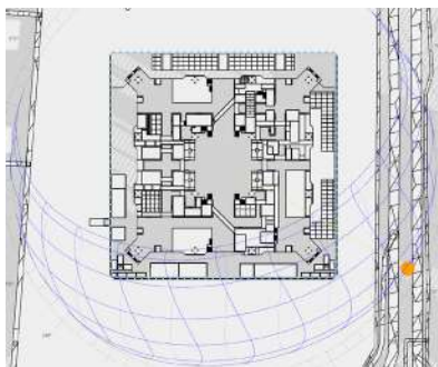
Figure 5.133: Winter solstice solar penetration at 09:00
