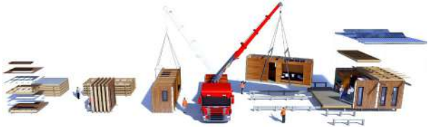
Figure 0.6: installation procedure transition from flat panel components to fully enclosed volumetric block.
