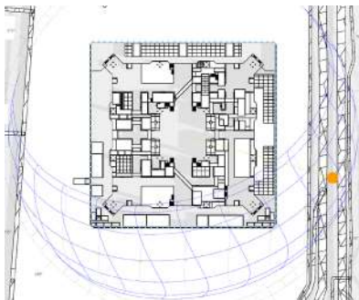
Figure 5.130: Autumnal equinox solar penetration at 09:00
