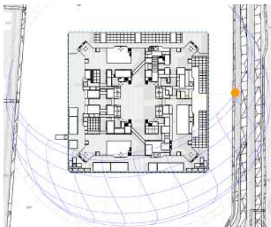
Figure 5.127: Summer solstice solar penetration at 09:00
