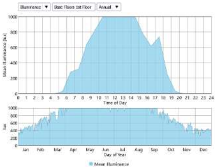
Figure 5.73: Base illuminance chart first floor.
