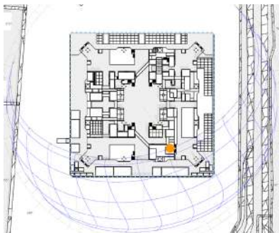
Figure 5.128: Summer solstice solar penetration at 12:00
