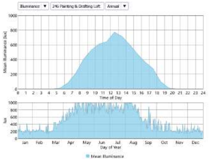
Figure 5.143: Workshop illuminance chart first floor south perimeter.
