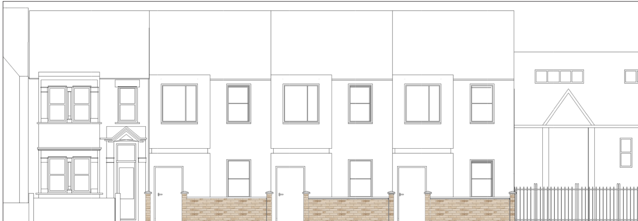
Figure 5.23 Material application on the proposed street elevation, showing the use of light buff facing brick as an entrance border to frame the access points, define the threshold, and introduce subtle material variation within the façade . (Author's drawing.)
