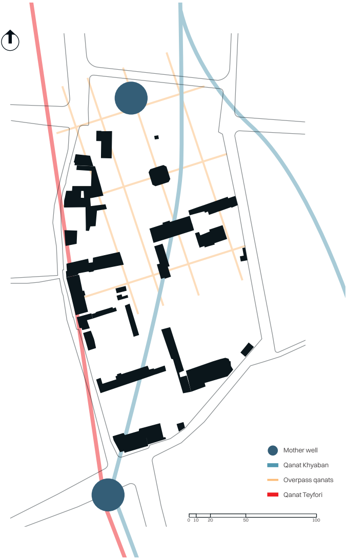
Figure.64 Qanat system, Effects the Garden directly.
