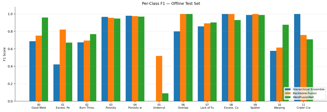
Figure 6.2: Per-class F1 for all three models on the offline final 12-class test set (780 runs). Class 05 (undercut) is the principal failure mode across approaches, and class 10 (warping) is the secondary one. WeldFusionNet leads on the head classes (good weld, lack of fusion, warping); Backbone Fusion distributes performance more evenly and leads on macro-F1 by partially recovering classes 01 and 05.
