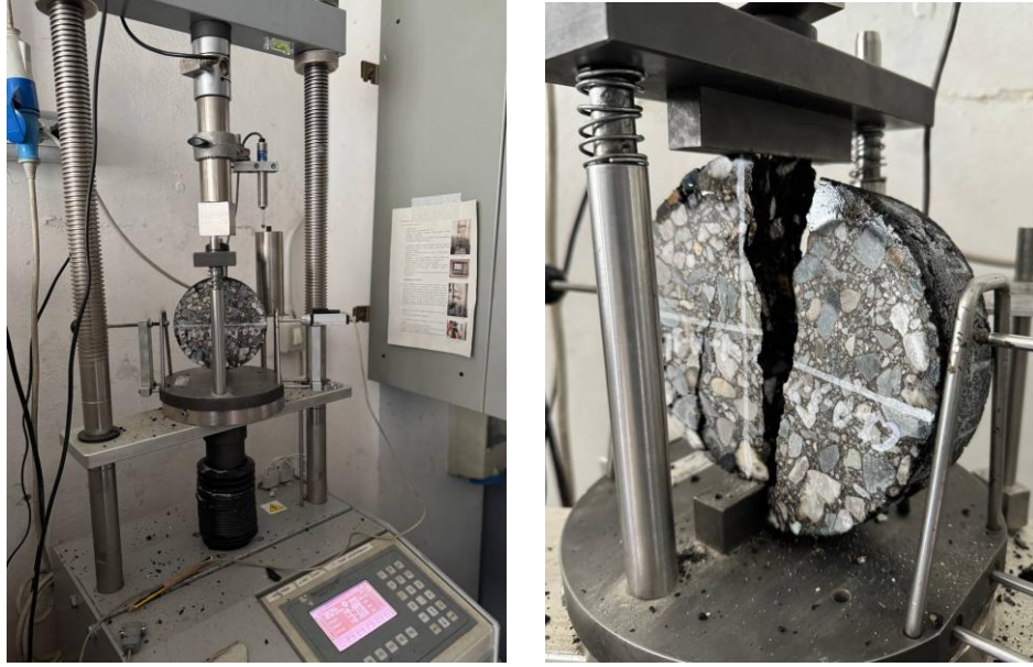
Figure 17- Indirect tensile strength test setup and typical diametral fracture of an asphalt mixture specimen after testing.
