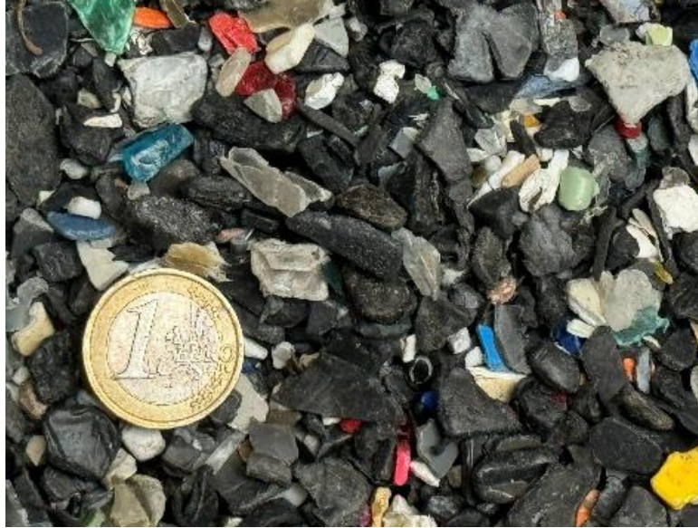
Figure 5 – Recycled-plastic material M selected for incorporation into the asphalt mixtures.
