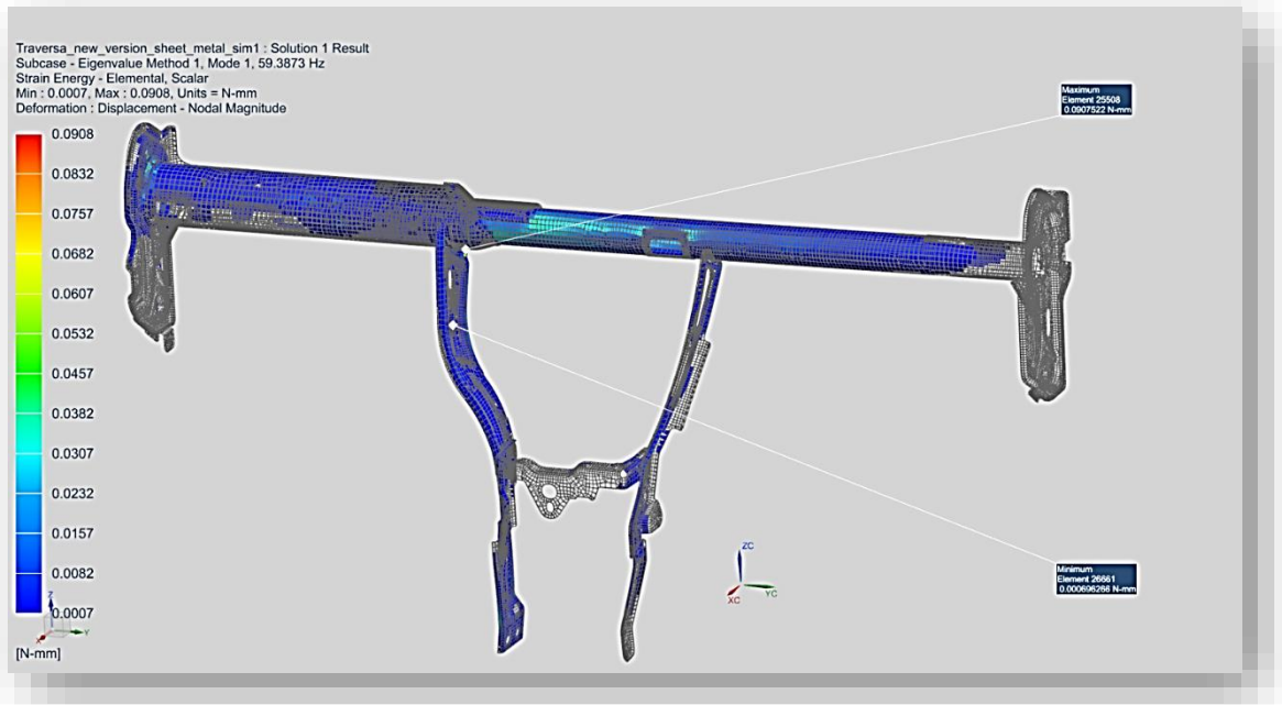
Figure 5.51 Strain energy distribution of mode 1 for the proposed CCB model
