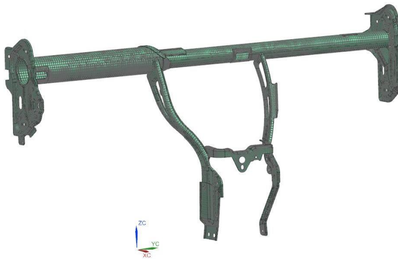
Figure 4.47 Finite element mesh generated for the proposed CCB model
