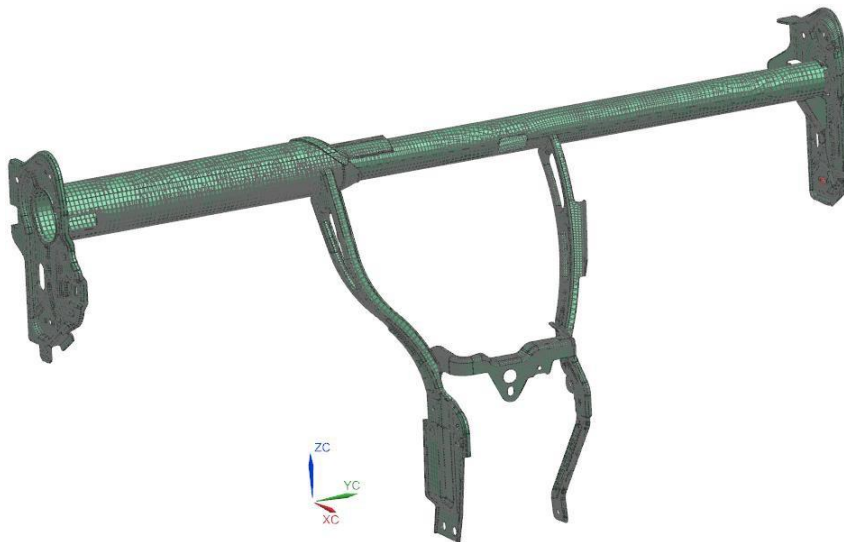
Figure 4.46 Finite element mesh generated for the optimized CCB model
