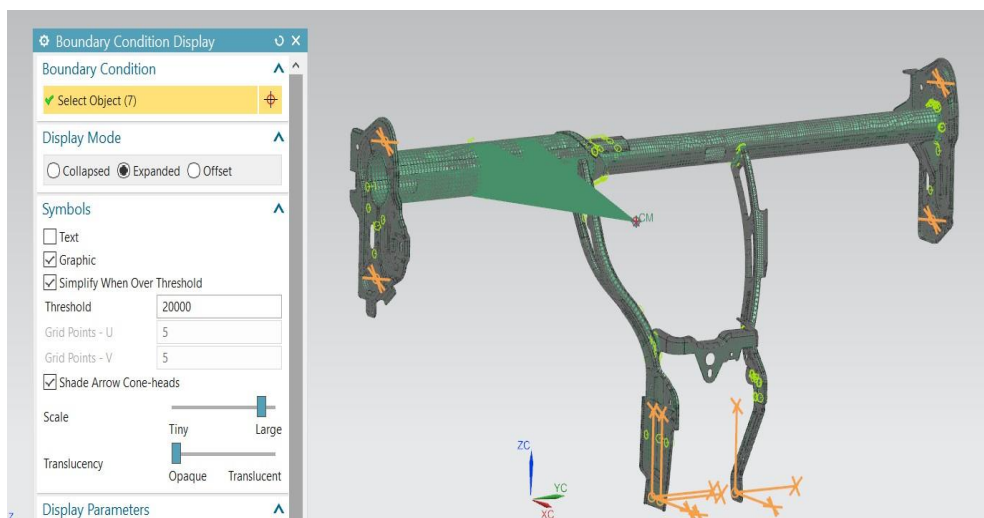
Figure 4.63 Boundary conditions applied to the optimized CCB model
