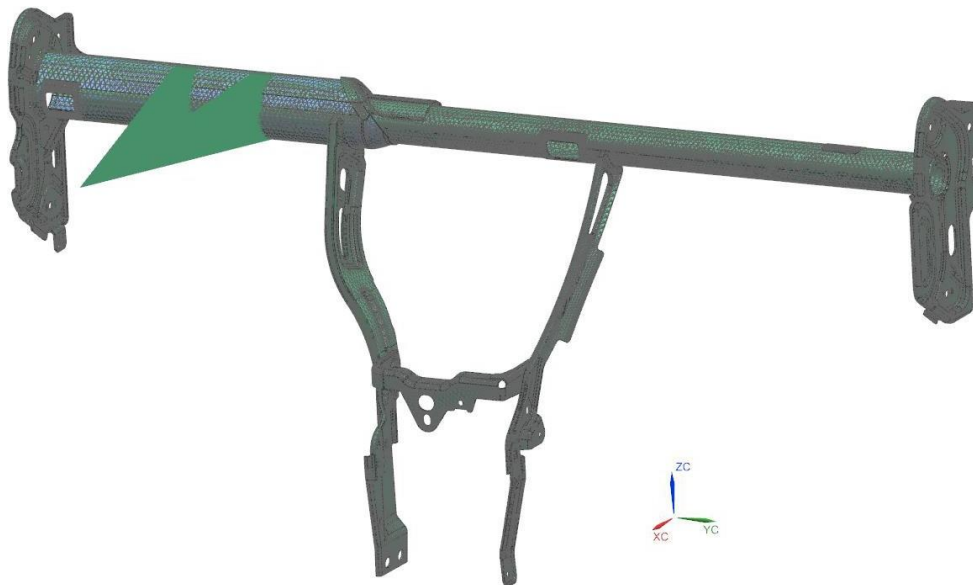
Figure 4.32 RBE 2 applied for the Steering wheel column on proposed Cross-Car Beam model
