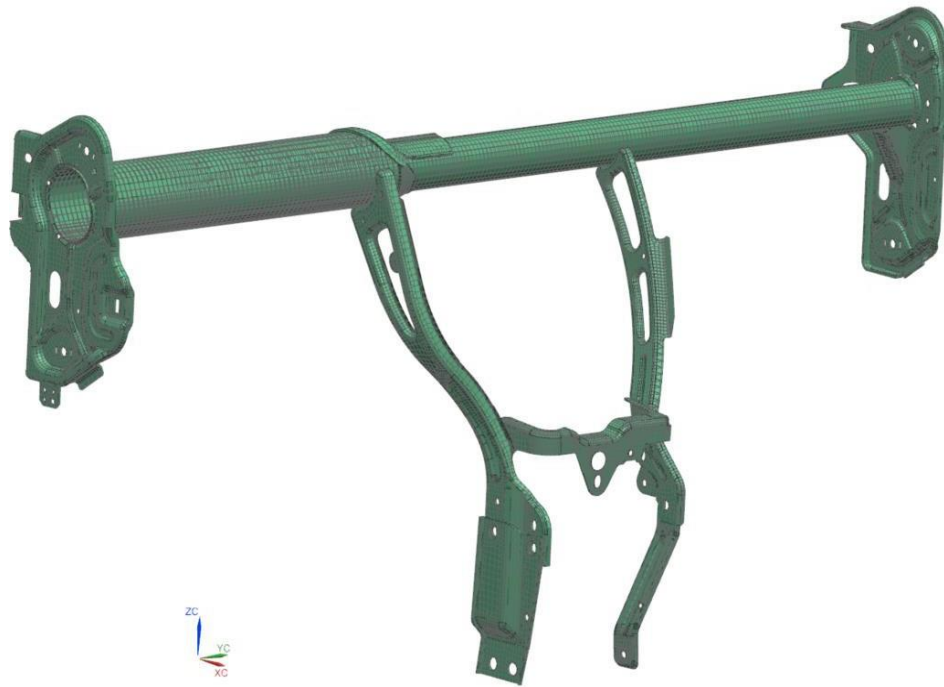
Figure 2.10 Finite element mesh model of the Cross-Car Beam assembly
