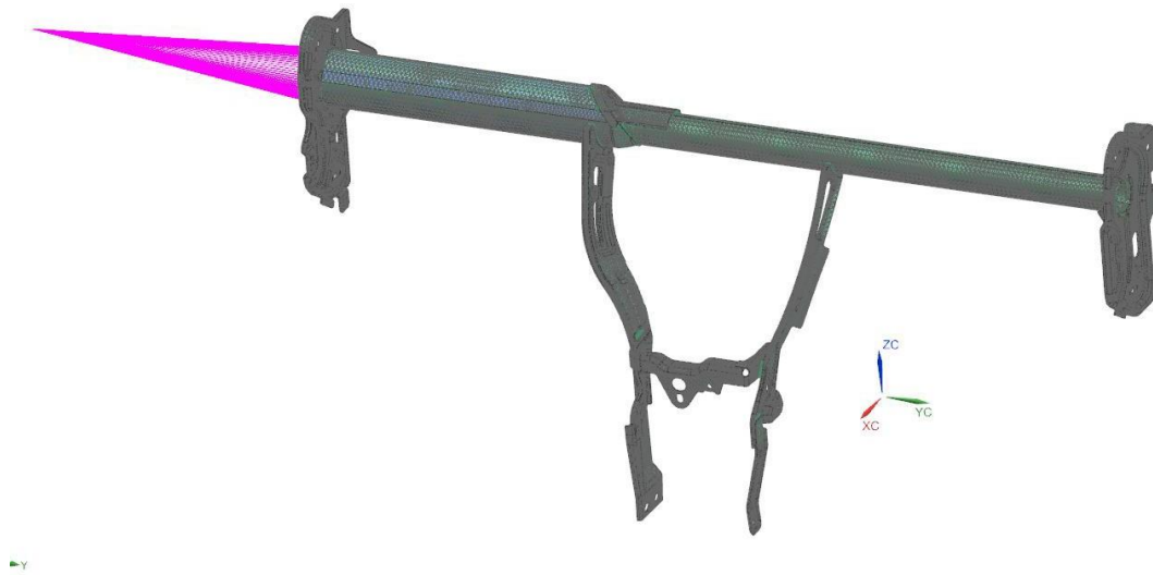
Figure 4.21 RBE 3 configurations (pink) applied on solid Cross-Car Beam model 450mm distance from A-pillar
