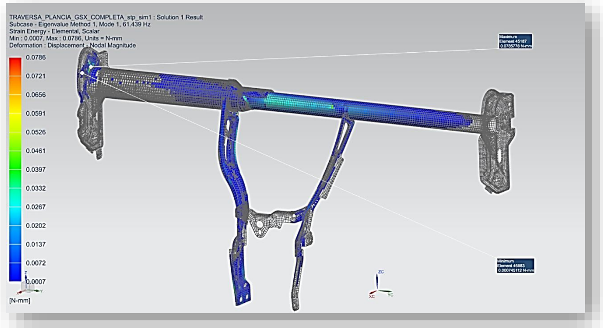
Figure 5.39 Strain energy distribution of mode 1 for the solid CCB model
