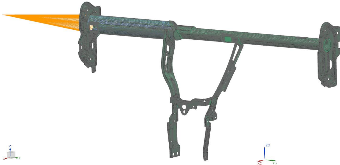
Figure 4.23 RBE 3 configurations (orange) applied on proposed Cross-Car Beam model 450mm distance from A-pillar
