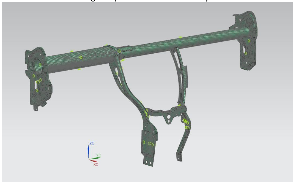
Figure 4.48 Glue connections and mesh mating definitions applied to the solid CCB model marked as yellow
