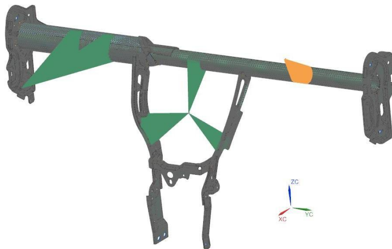
Figure 4.36 RBE 2 applied for the Airbag unit on solid Cross-Car Beam model marked as orange
