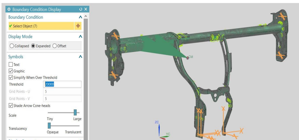
Figure 4.64 Boundary conditions applied to the proposed CCB model
