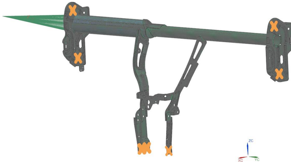
Figure 4.27 Constraints are applied to the solid Cross-Car Beam marked as orange
