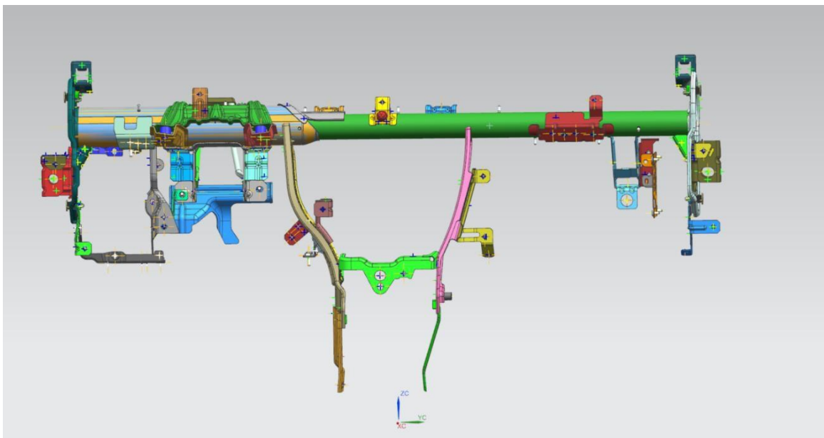
Figure 4.1 Original solid Cross-Car Beam model used as the reference configuration
