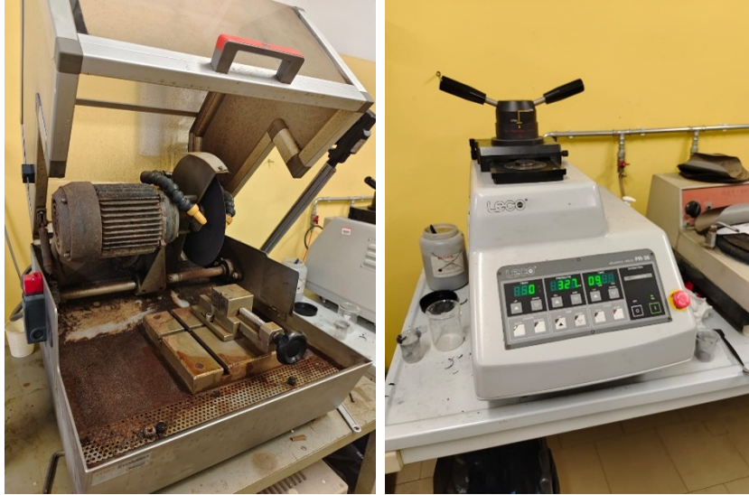
Figure 3.1: a) Precision abrasive cut saw. b) LECO PR-63 Mounting press for embedding.
