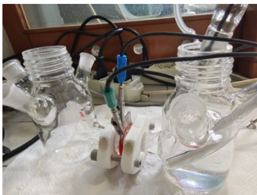
Figure 3.7: Permeation Cell showing the Working electrode (Alloy sample) in between the Anodic compartment (Right) and the cathodic compartment (Left).
