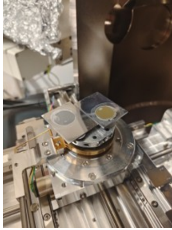
Figure 3.9: Alloy samples mounted on a sample holder to be observed under the FESEM.
