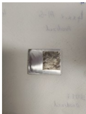
Figure 3.6: Palladium coated region on Al-6016 sample.
