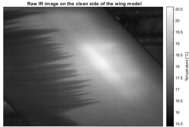
Figure 2.7: Saw-tooth transition front produced by stationary crossflow vortices. Captured by infrared thermography on the clean side of the wing model during the experimental campaign. The forcing is generated by 12 mm spaced DREs located only in the middle span, as it can be seen by the transition delay in the spanwise extremities; the flow goes from right to left.
