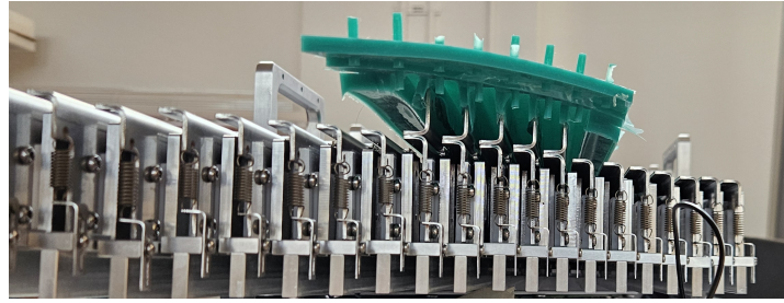
Figure 3.8: Assembly of the skin and the mechanical actuators using an experimental green skin composed of only five legs.
