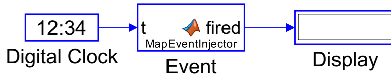
Figure 7.1: MapEventInjector MATLAB fcn block: Digital Clock provides simulation times, the generated event is shown with a flag in Display block. Located at swarm_phase_5 .
