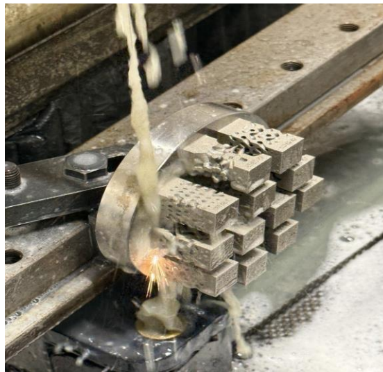
Figure 26. Separation of LPBF-fabricated Stainless Steel 316L Lattice Specimens from the Build Platform Using WEDM.
