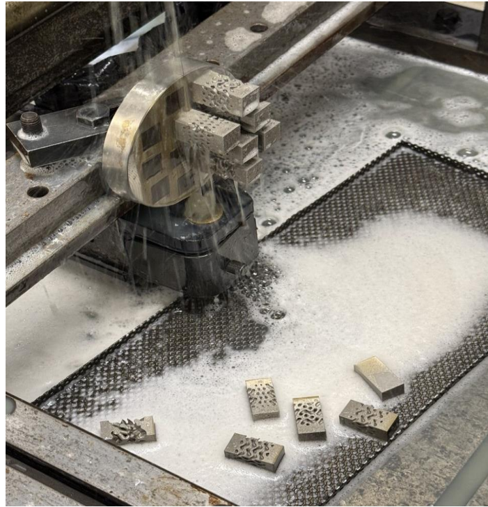
Figure 17. Lattice Separation from Build Platform using WEDM [Image taken during specimen preparation].
