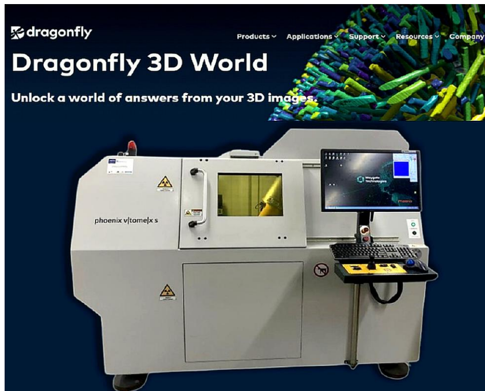
Figure 28. The Dragonfly Software Used to Analyze the XCT Data and the Phoenix v|tome|x S XCT System Used to Acquire the Data [88].
