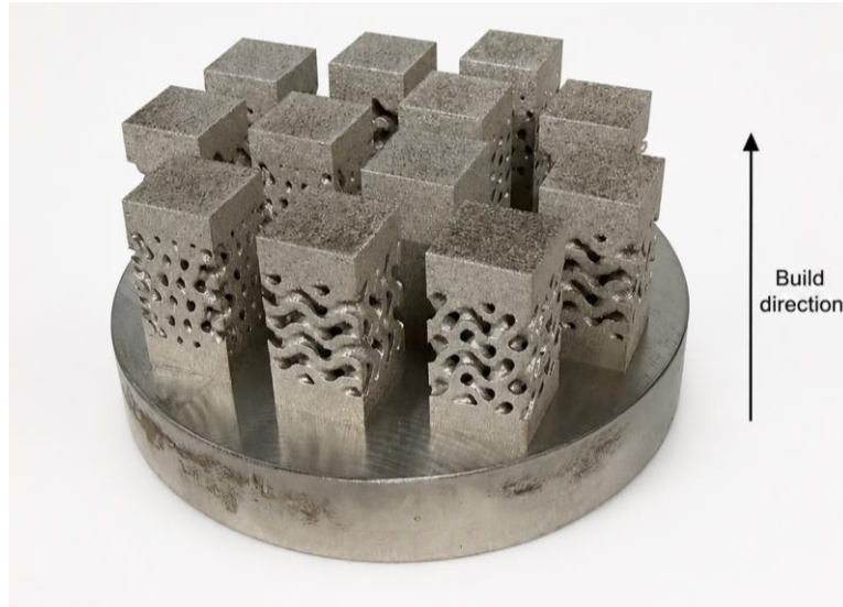
Figure 25. Printed Build Platform Containing the Stainless Steel 316L Compression Specimens Fabricated by LPBF.
