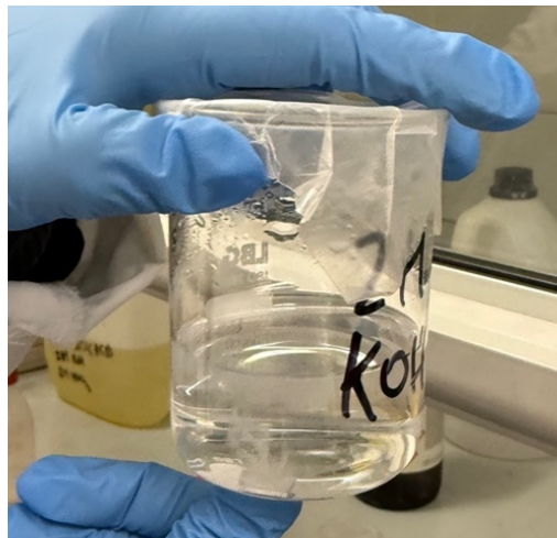
Figure 19. Immersion of an Al6016 specimen in the KOH solution during alkaline surface treatment before brazing
