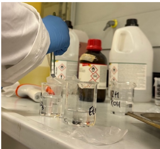
Figure 20. Immersion of an Al6016 specimen in the HNO 3 solution during acid surface treatment before brazing
