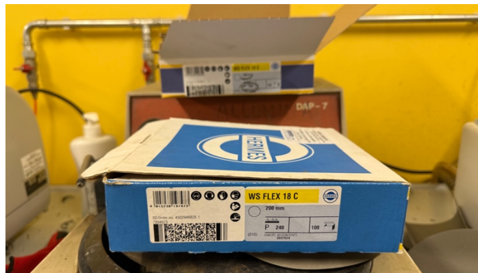
Figure 31. P240 waterproof SiC abrasive paper box used in the first grinding step
