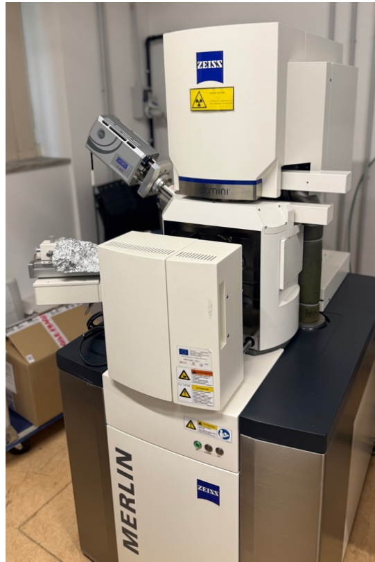
Figure 42. Zeiss Merlin field-emission scanning electron microscope equipped with Gemini column, used for backscattered electron imaging
