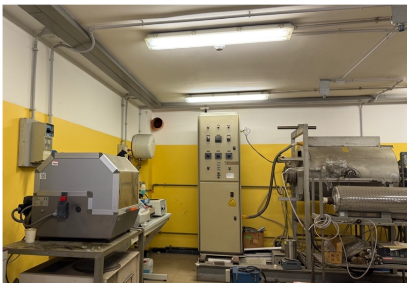
Figure 14. Laboratory equipment for sample preparation - Cutting (Remet TR80 Evolution) and Grinding/Polishing machines used for metallographic preparation
