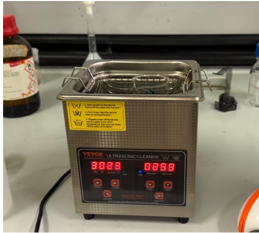
Figure 21. Ultrasonic bath used for ethanol cleaning of the specimens, with a beaker placed inside the bath during the cleaning step
