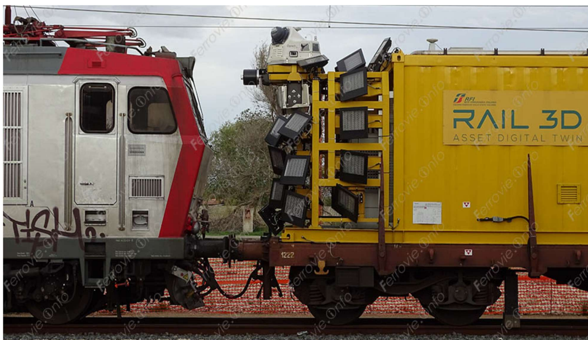
Figura 10: Carro diagnostico RAIL 3D "Asset Digital Twin".
