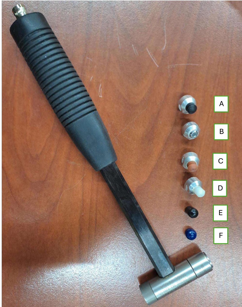
Figure 4.1: The Hammer, the tips and the covers available in the Lab, A ( Soft Impact Tip), B (Hard Impact metallic Tip), C ( Super soft Impact Tip), D (Medium Impact Tip) , E,F (Tip covers, only for tip protection)
