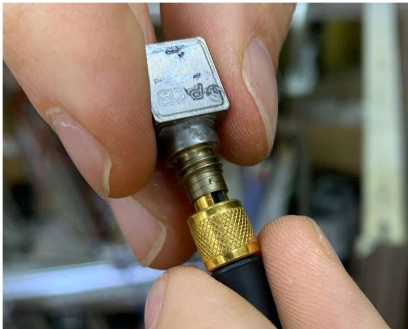
Figure 5.1: PCB 356A45 tri-axial accelerometer
