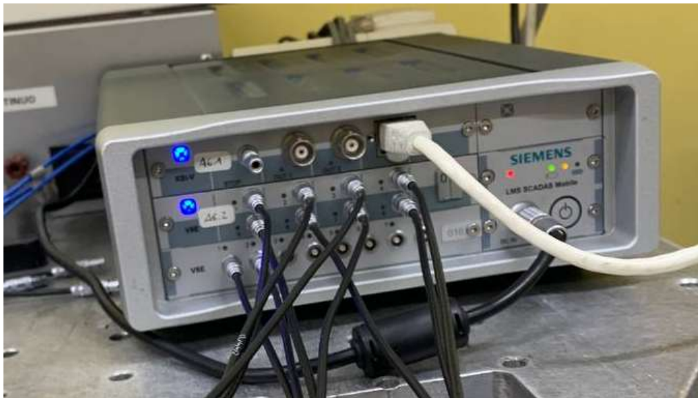
Figure 5.3: SCADAS acquisition system
