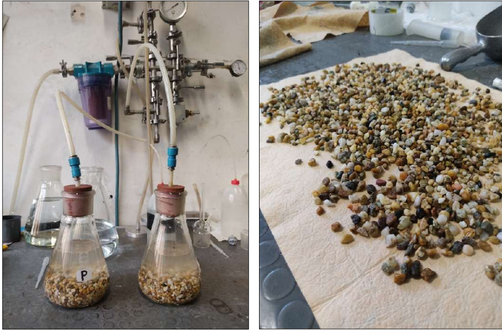
Figure 3.2: Laboratory procedure for determining the particle density and water absorption of aggregates in accordance with EN 1097-6: (a) vacuum de-airing of submerged samples within pycnometer flasks, and (b) conditioning of coarse aggregate particles to a Saturated Surface Dry (SSD) state
