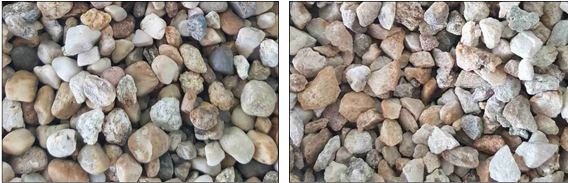
Figure 3.1: Morphological profiles of (a) Risino (100% rounded aggregate) exhibiting smooth geometry coarse aggregate fractions, and (b) Graniglia (100% crushed aggregate) displaying high angularity and surface roughness (adapted from Cave Germaire).
