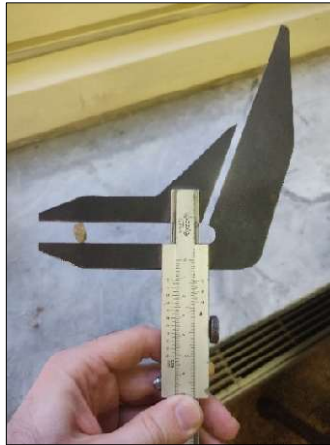
Figure 3.4: Evaluation of coarse aggregate particle elongation using a specialised calliper in accordance with EN 933-4.
