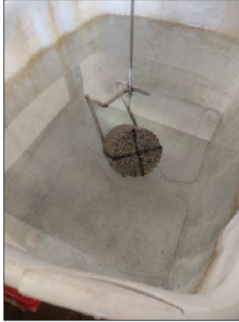
Figure 3.10: Submerged weighing of a cured porous concrete specimen to determine its immersed mass ( W_s ) during porosity validation.
