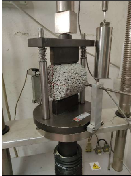
Figure 3.11: Indirect tensile strength (ITS) testing of a cured porous concrete specimen on the 7 th day of curing.
