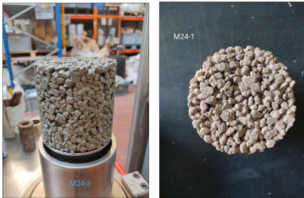
Figure 5.1: The M24 mix design in its fresh and cured states
