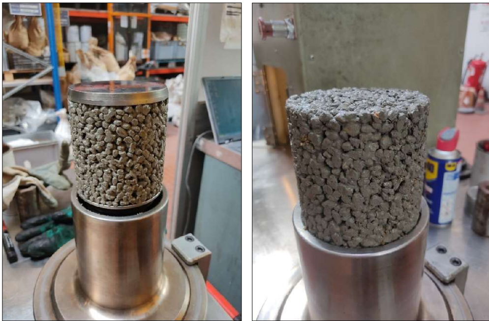
Figure 3.8: Freshly extruded porous concrete specimen following gyratory compaction, prepared for transfer to the moisture-controlled curing chamber.
