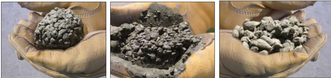
Figure 1.1: Subjective visual assessment of fresh porous concrete workability using the qualitative manual hand-ball test under varying water contents (adapted from Tennis et al., 2004)
