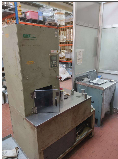
Figure 1.3: The standard Superpave Gyratory Compactor equipment and integrated data-acquisition system used to characterise fresh-state porous concrete compaction indices
