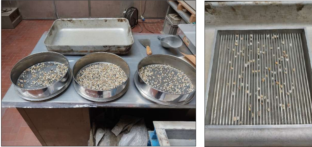
Figure 3.3: Laboratory procedure for determining the Flakiness Index (FI) of coarse aggregate fractions in accordance with EN 933-3: (a) mechanical separation into size sub-fractions, and (b) thickness gauging using parallel bar sieves.
