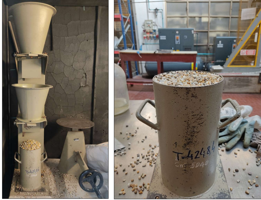
Figure 3.5: Laboratory test configuration for determining the uncompacted (loose) bulk density and void content of coarse aggregate fractions in accordance with EN 1097-3.
