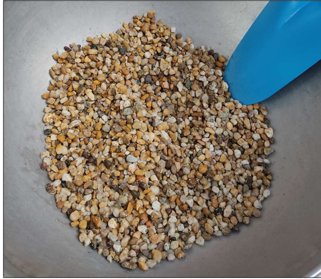
Figure 3.6: Coarse and fine aggregate batch prepared in the Saturated Surface Dry (SSD) state prior to the mixing phase.
