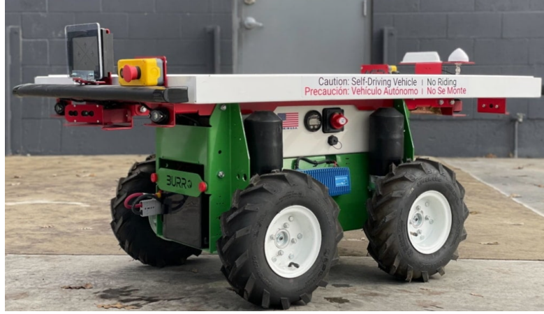
Figure 2.4: The Burro 8.2 collaborative agricultural carrier. Source: Augean Robotics (via Agtecher) [14].
