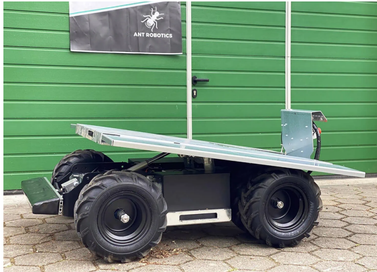
Figure 2.3: The Ant Robotics Adir Power , a four-wheel electric carrier for transport and maintenance in orchards and vineyards. Source: Ant Robotics (via Future Farming) [13].
