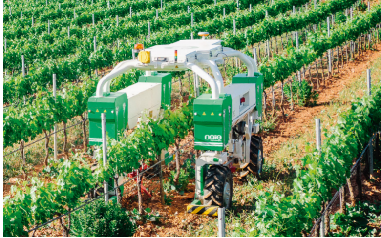
Figure 2.2: The Naïo Technologies Ted straddle robot for autonomous weeding and canopy management in vineyards. Source: Naïo Technologies [5].
