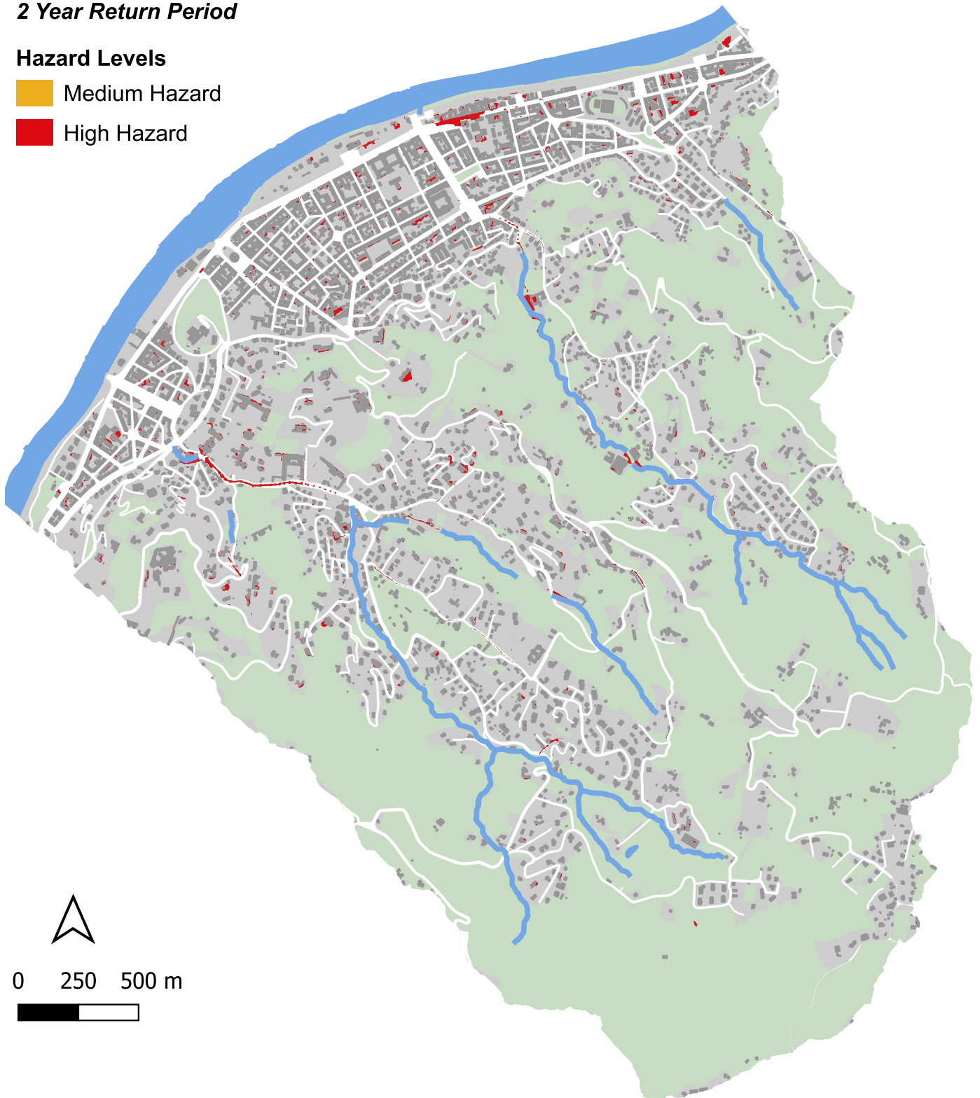
Figure B.1: Pedestrian flood hazard map for a return period of 2 years.
