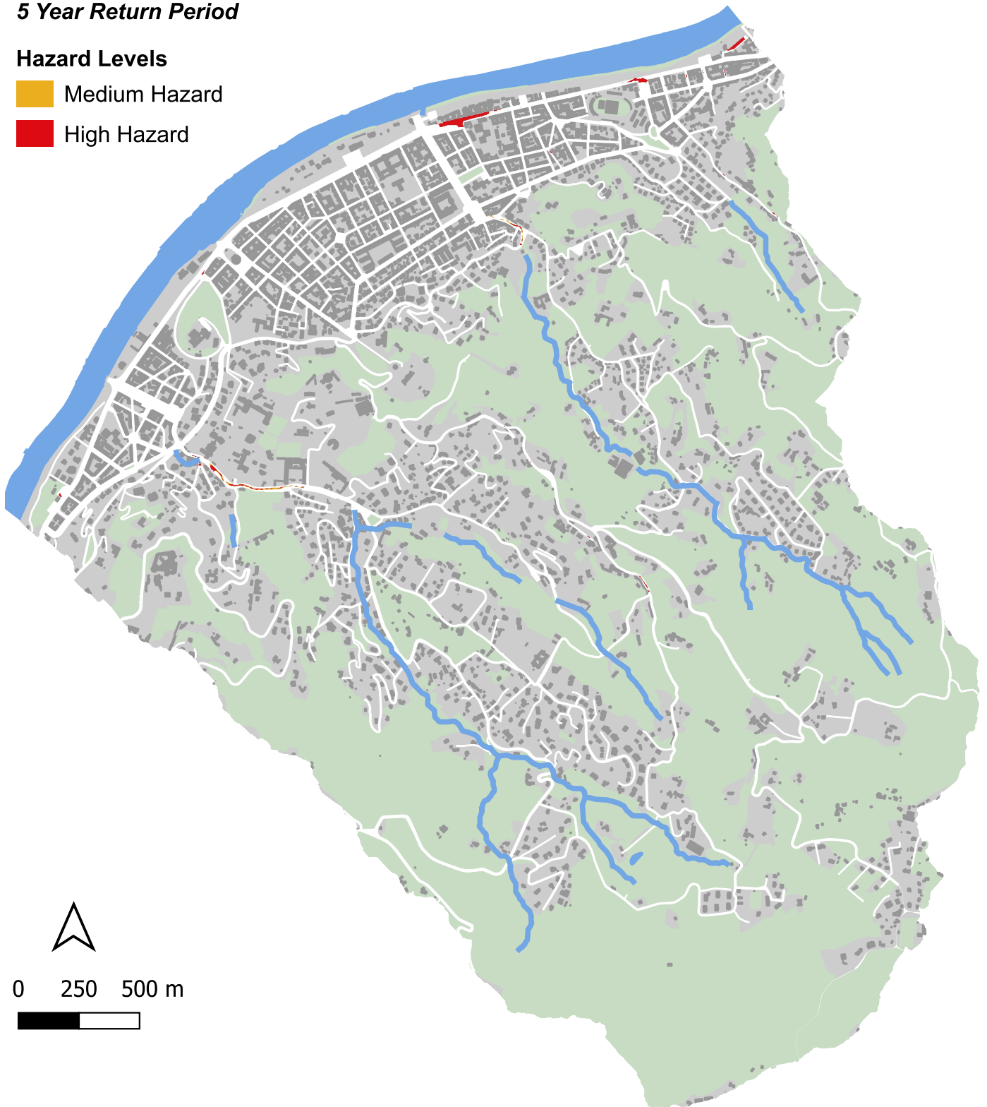
Figure B.7: Vehicular flood hazard map for a return period of 5 years.
