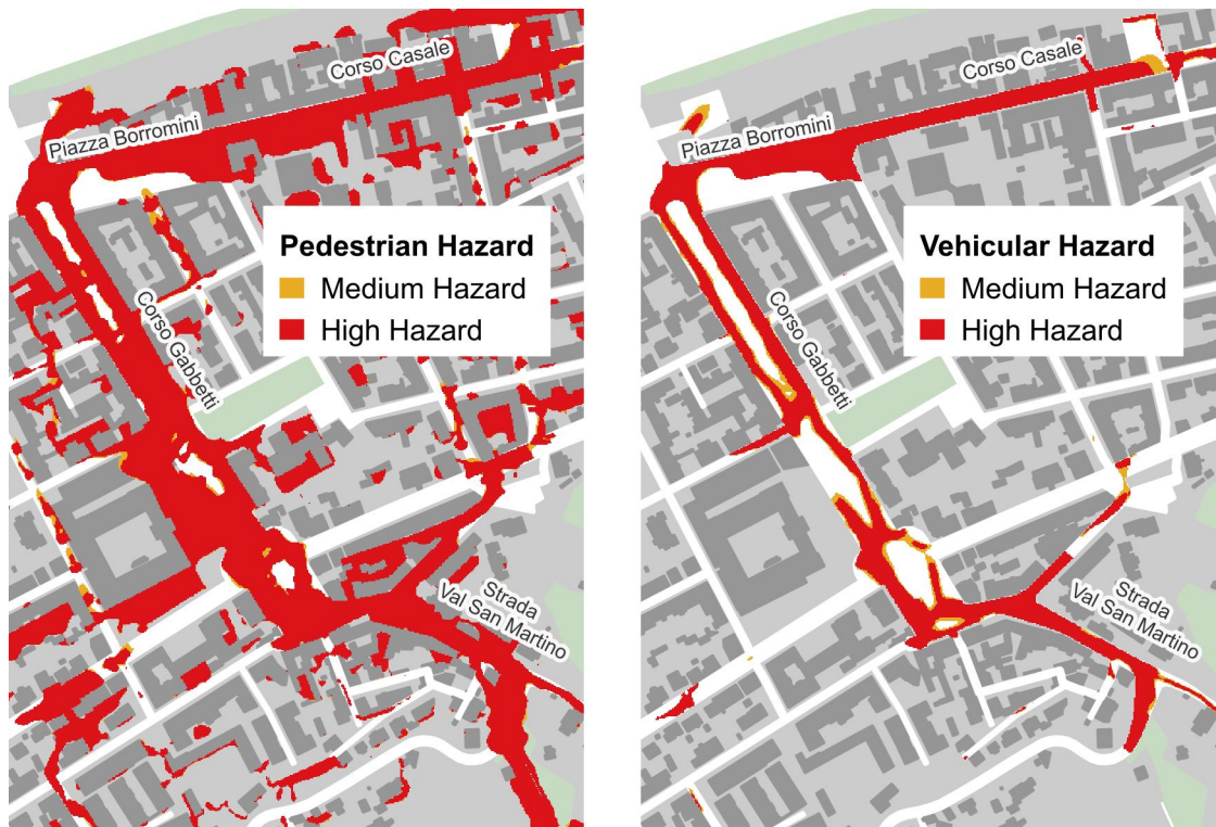
Figure 5.4: Pedestrian and vehicle hazard levels ( T_r = 100 years) in the area affected by the flooding of Rio Val San Martino.
