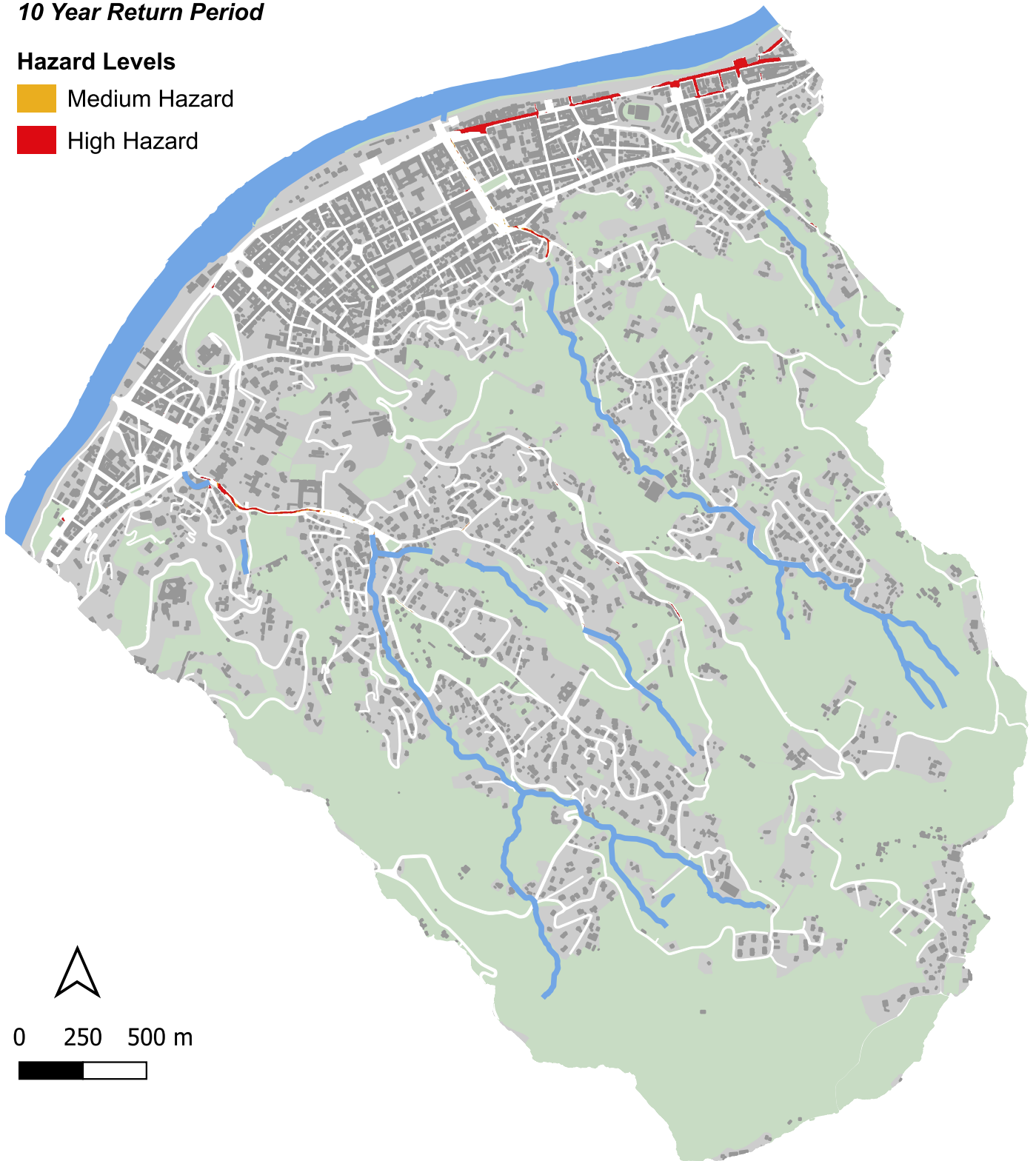
Figure B.8: Vehicular flood hazard map for a return period of 10 years.
