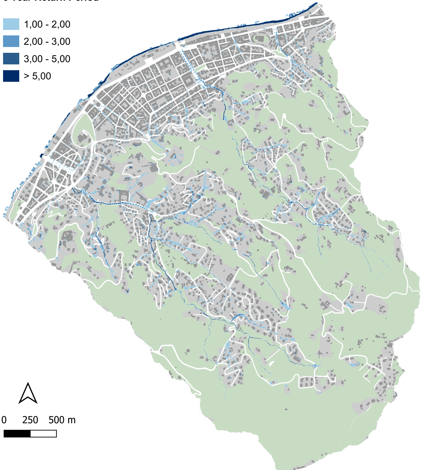
Figure A.7: Water velocity map for a return period of 5 years.
