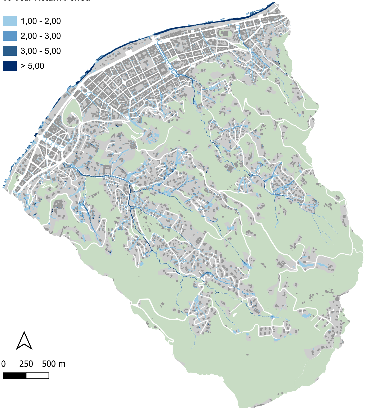
Figure A.8: Water velocity map for a return period of 10 years.
