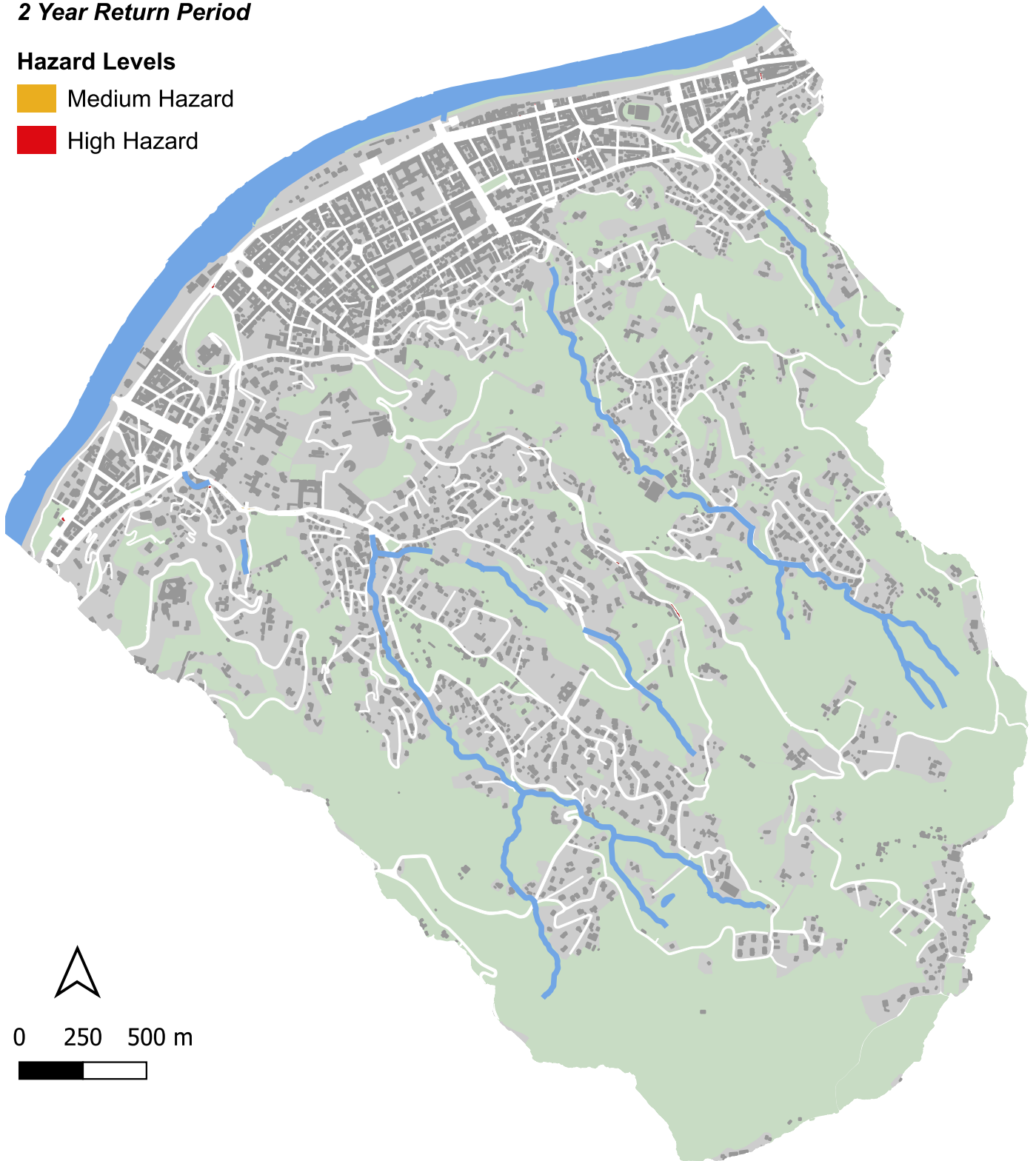
Figure B.6: Vehicular flood hazard map for a return period of 2 years.
