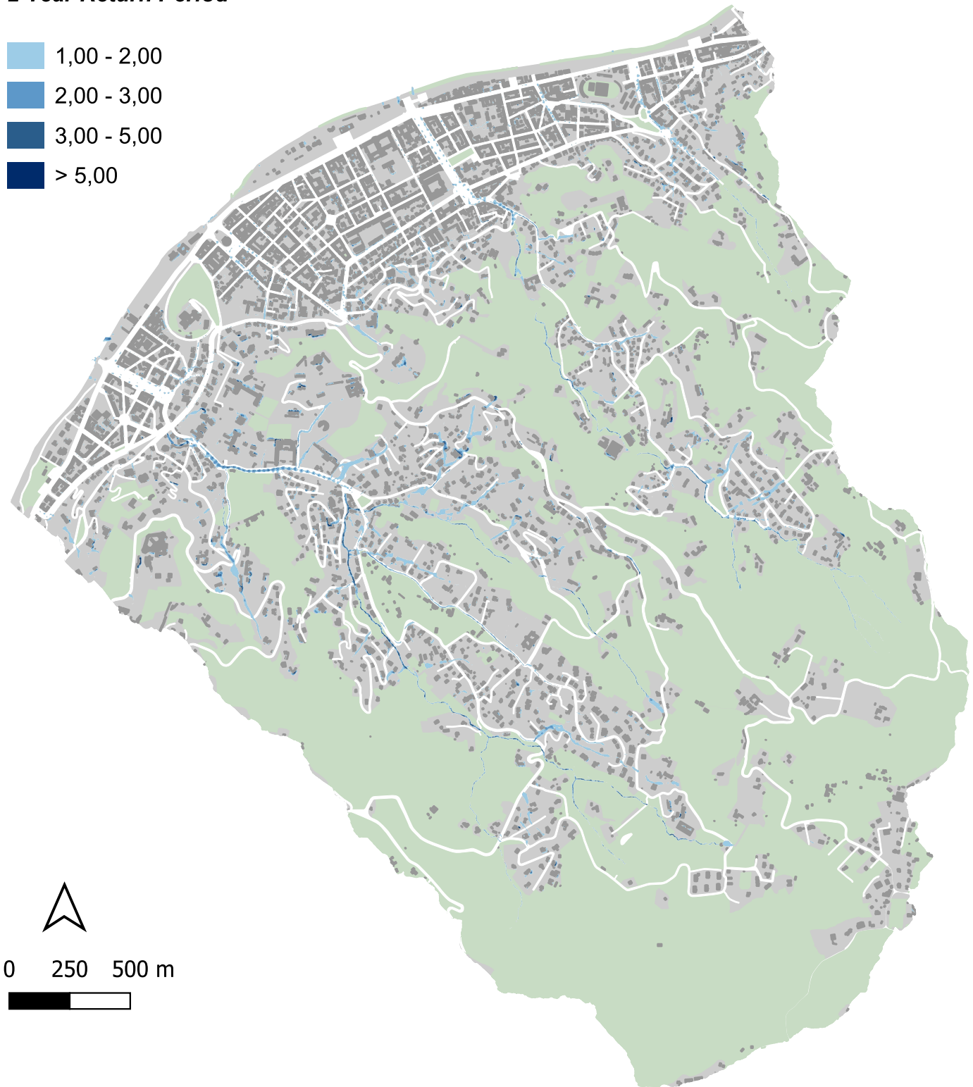
Figure A.6: Water velocity map for a return period of 2 years.
