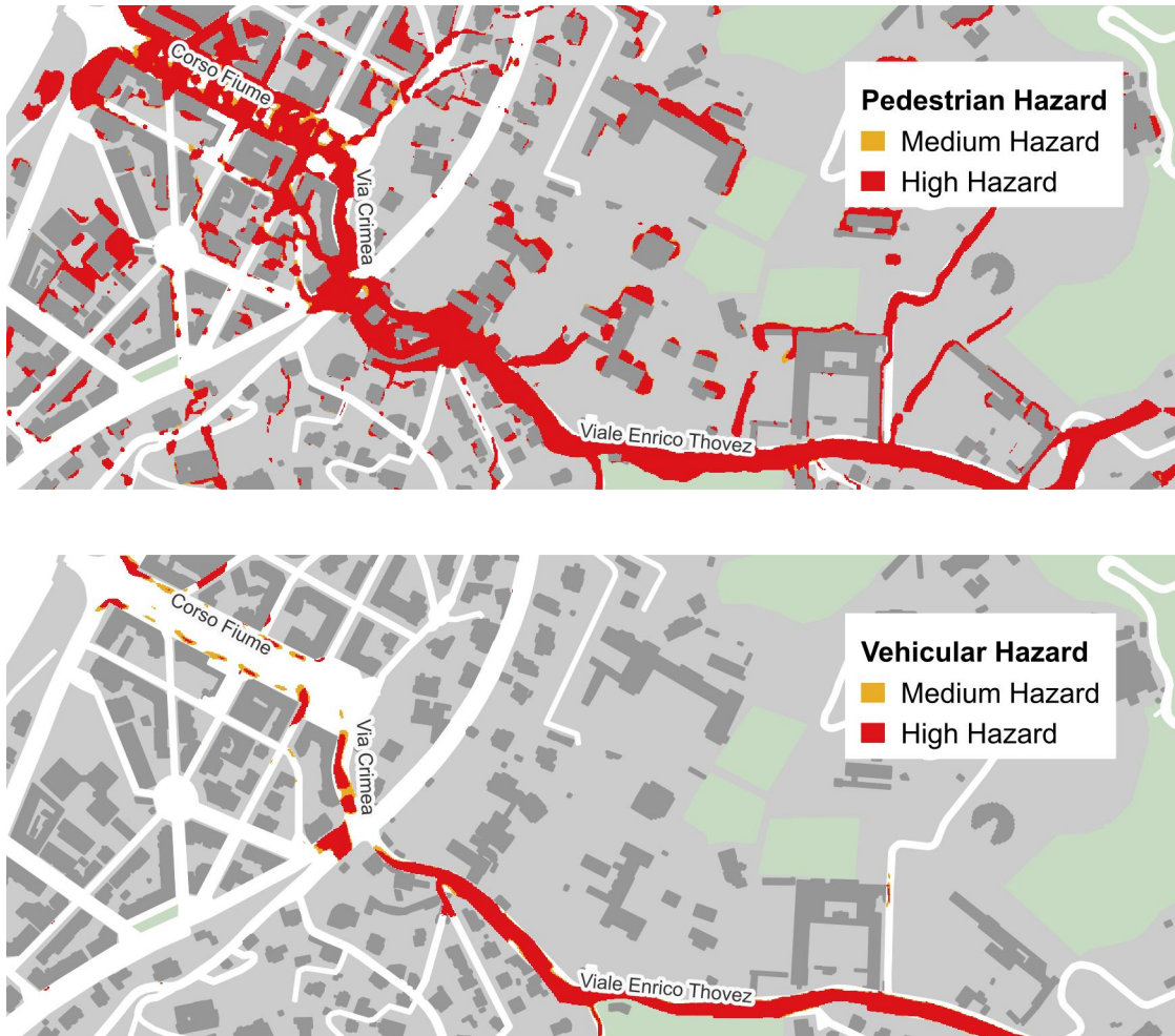
Figure 5.2: Pedestrian and vehicle hazard levels ( T_r = 100 years) in the area affected by the flooding of Rio Val Salice and Rio Pavese.
