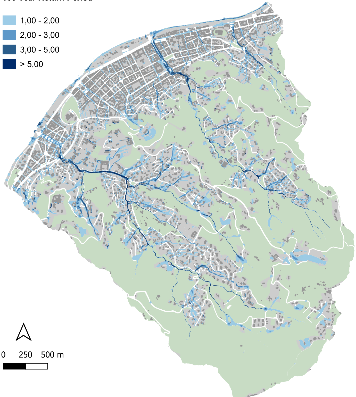
Figure A.9: Water velocity map for a return period of 100 years.
