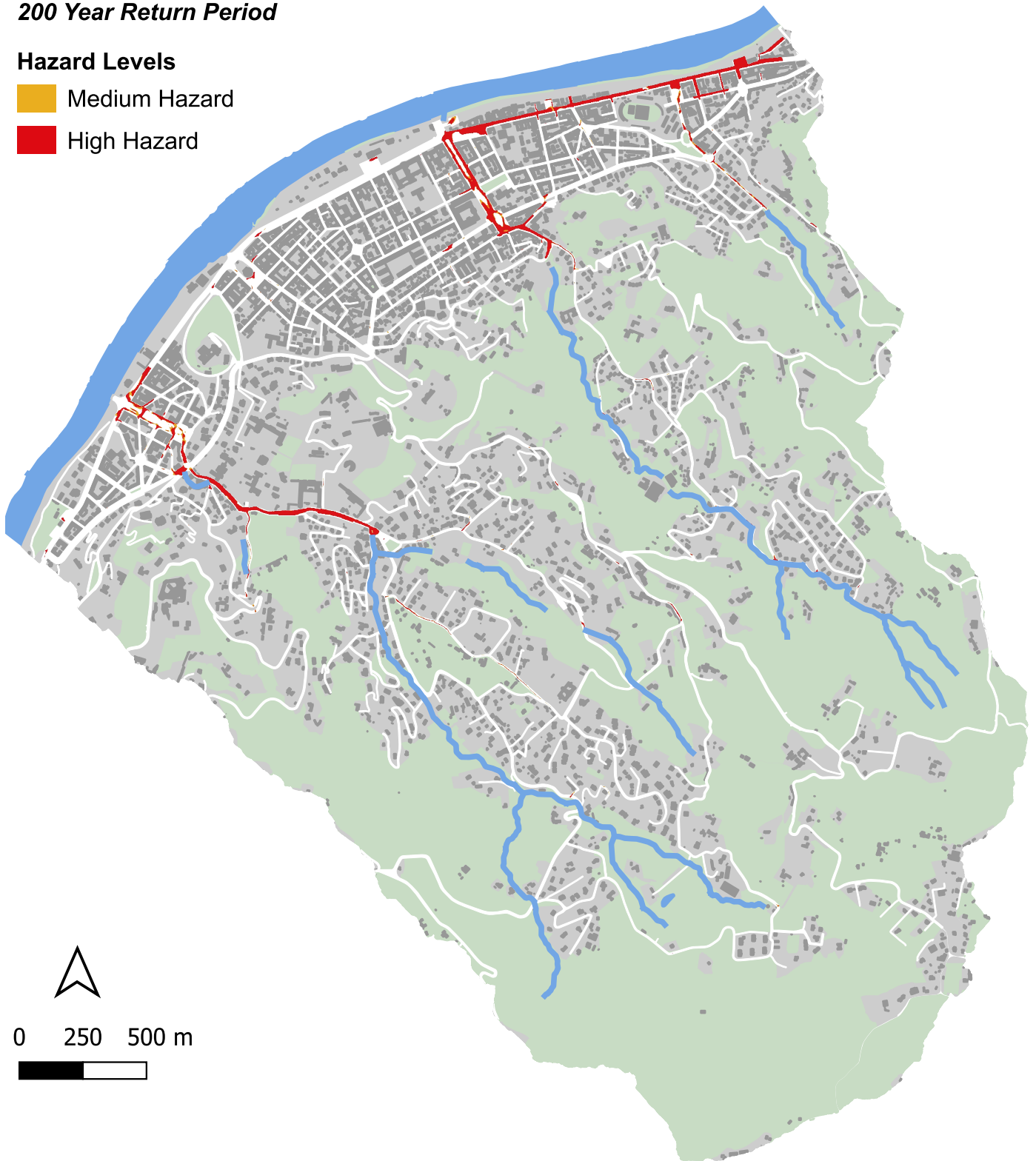
Figure B.10: Vehicular flood hazard map for a return period of 200 years.
