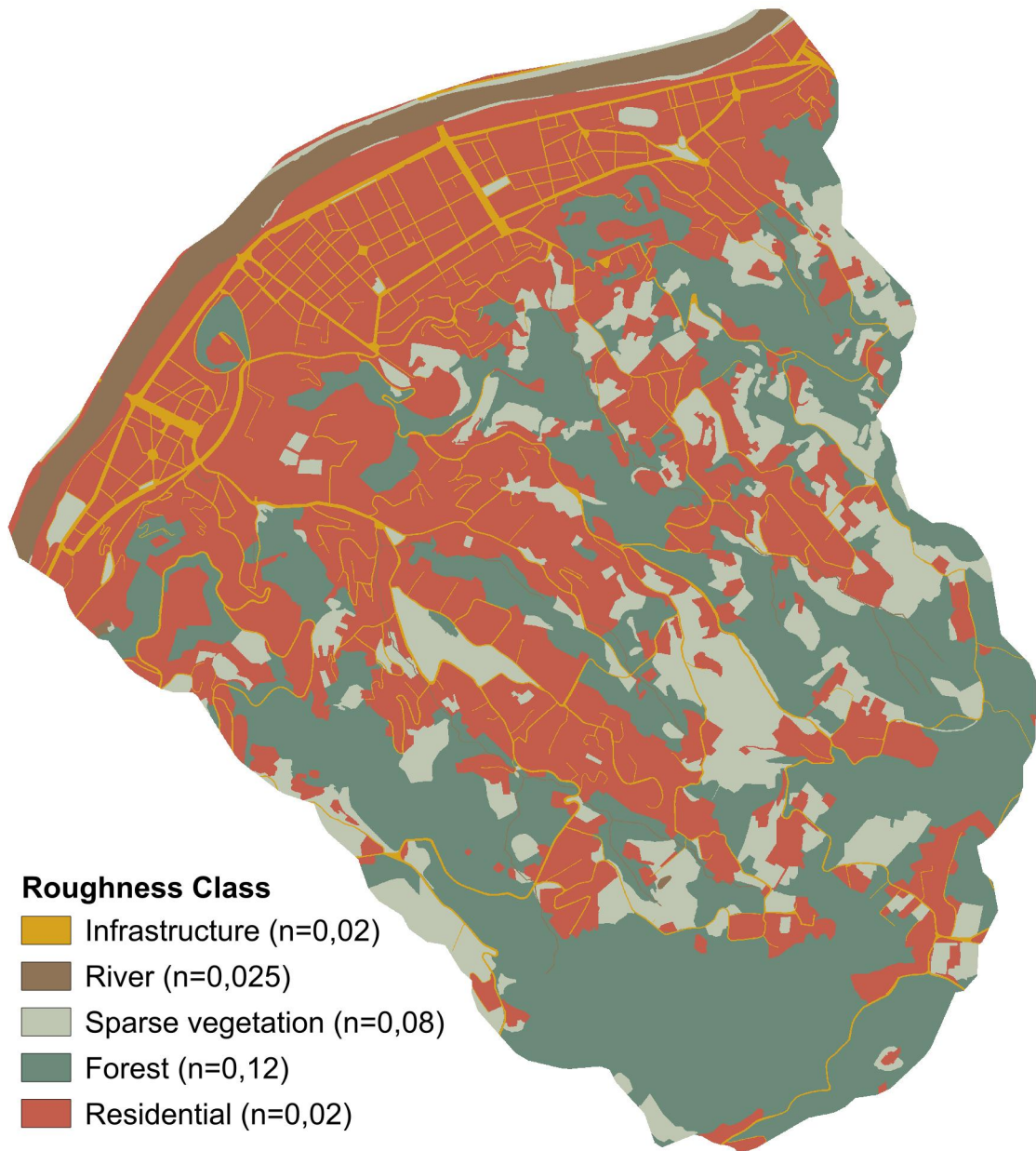
Figure 2.2: Spatial distribution of surface roughness classes across the catchment domain. Each zone is assigned a Manning's roughness coefficient.
