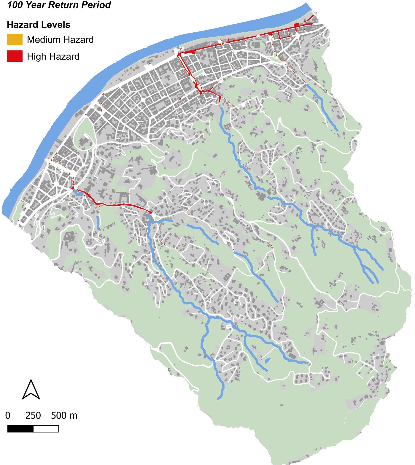
Figure B.9: Vehicular flood hazard map for a return period of 100 years.
