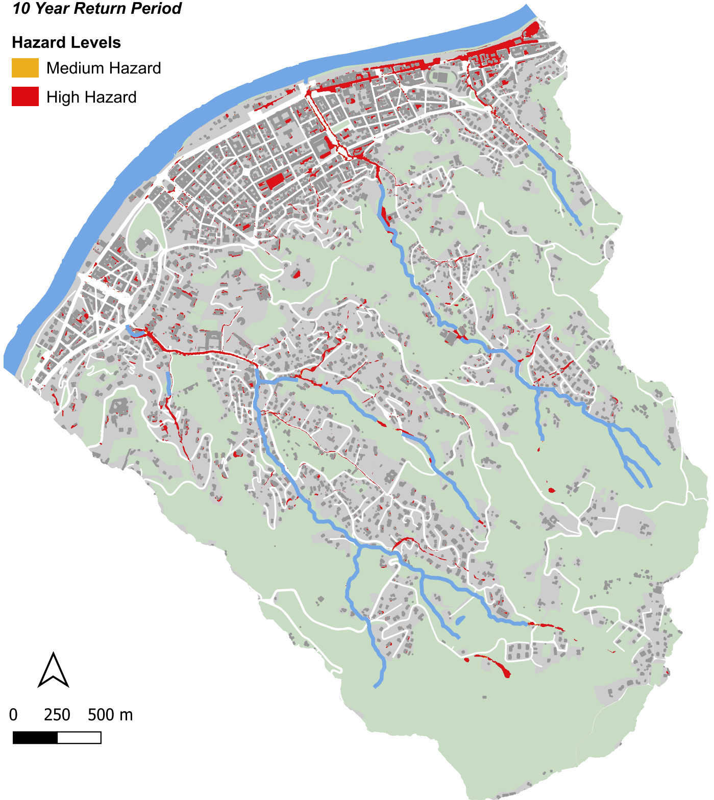
Figure B.3: Pedestrian flood hazard map for a return period of 10 years.
