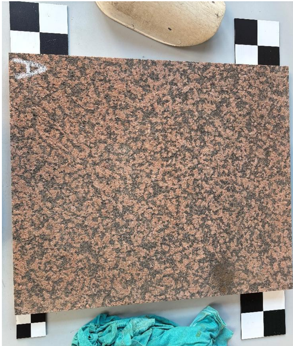
Figure 3.2: Configuration of rigid professional markers positioned on the outer vertices for metric alignment optimization.
