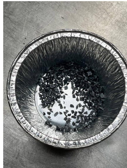
Figure 2.3.4-Dimension of plastic pellets after cutting
