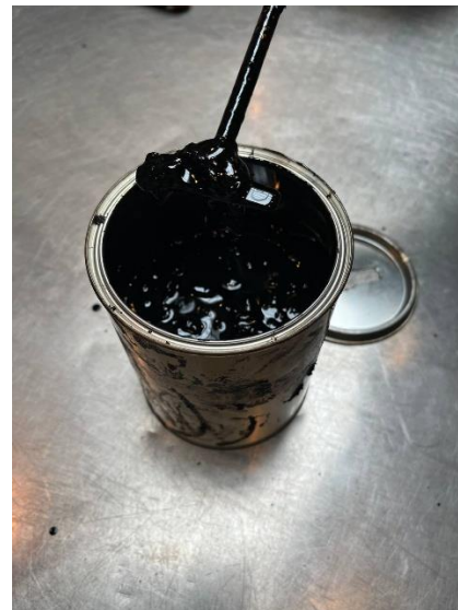
figure 2.3.2– unmelted plastics during mixing
