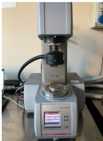
Figure 2.2.1 -Dynamic Shear Rheometer (DSR), MCR 302 Anton Paar
