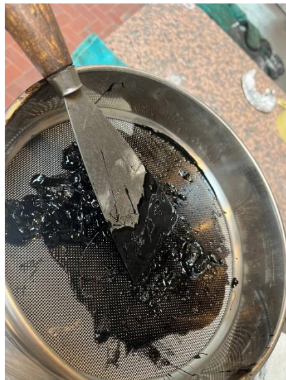
Figure 2.3.1 – plastics on sieve shows mixing failure
