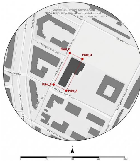
Figure 10 Topographic control network around the Energy Center building, showing the four exterior control stations (Points A–D). Basemap: Esri / OpenStreetMap.
