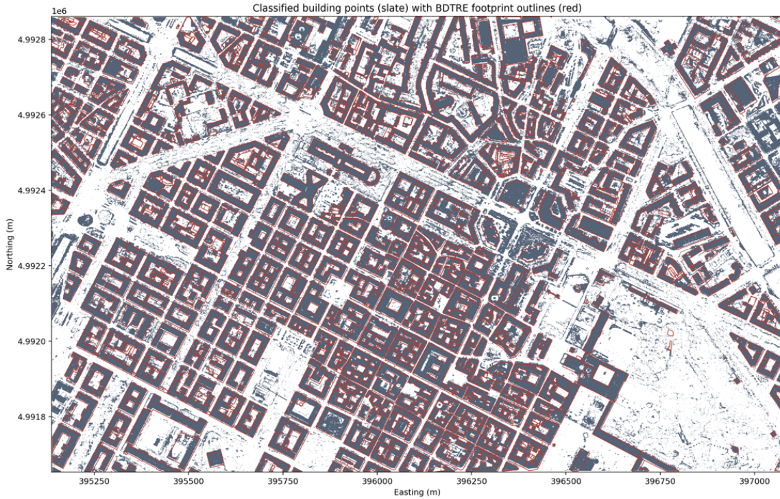
Figure 4.2: Inputs to the reconstruction: the classified building points (slate) with the BDTRE footprint outlines (red), over the study area.
