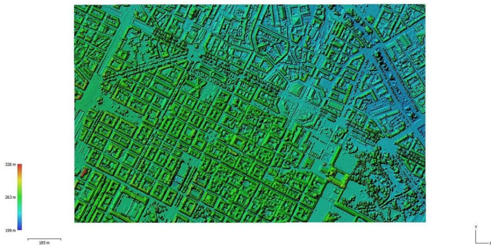
Figure 3.10: DSM generated from the Metashape classification. Vegetation wrongly kept as building introduces strong noise into the surface.
