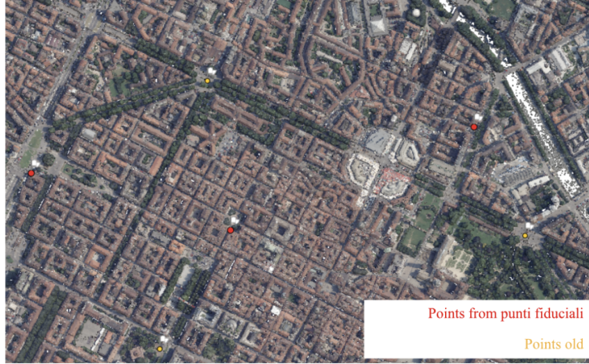
Figure 3.8: The three punti fiduciali selected from the Geoportale Piemonte dataset (Regione Piemonte, 2025), after coordinate transformation to WGS84 UTM 32N.
