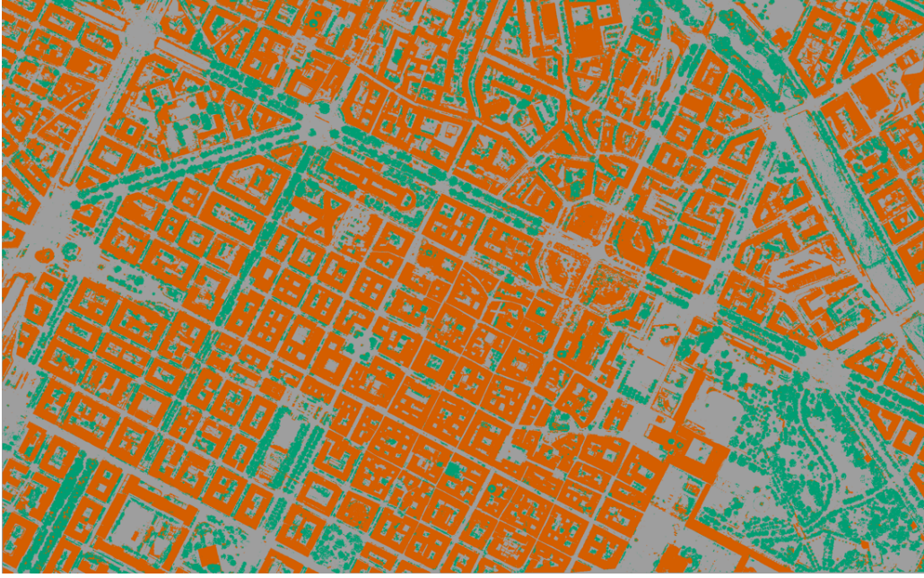
Figure 3.13: The full area after automatic classification, shown in a different viewer: here buildings are orange, trees green, and the ground grey.
