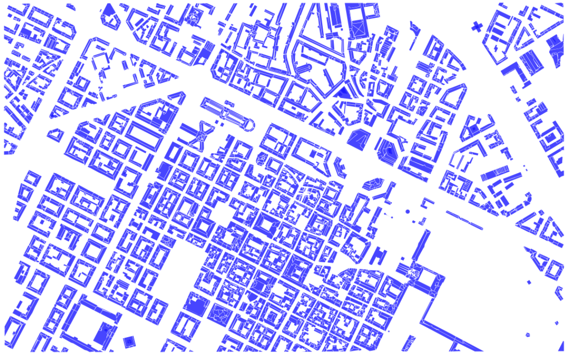
Figure 5.6: The LOD2.1 roof faces over the study area: 5434 planar faces reconstructed by geoflow-roofer. Each face is the unit onto which the classification is merged.
