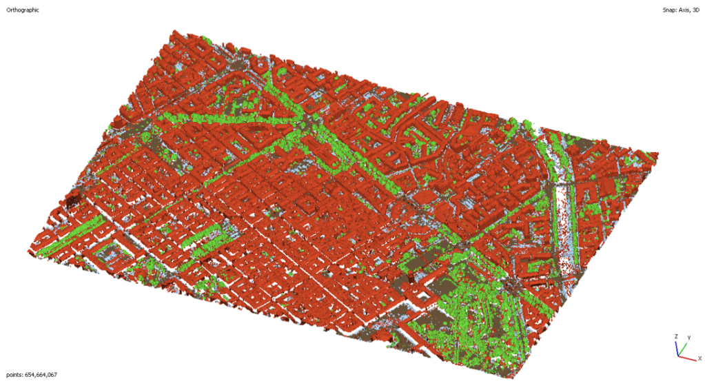
Figure 3.9: First classification attempt with the Metashape built-in tool (red = building, green = vegetation, blue = ground).
