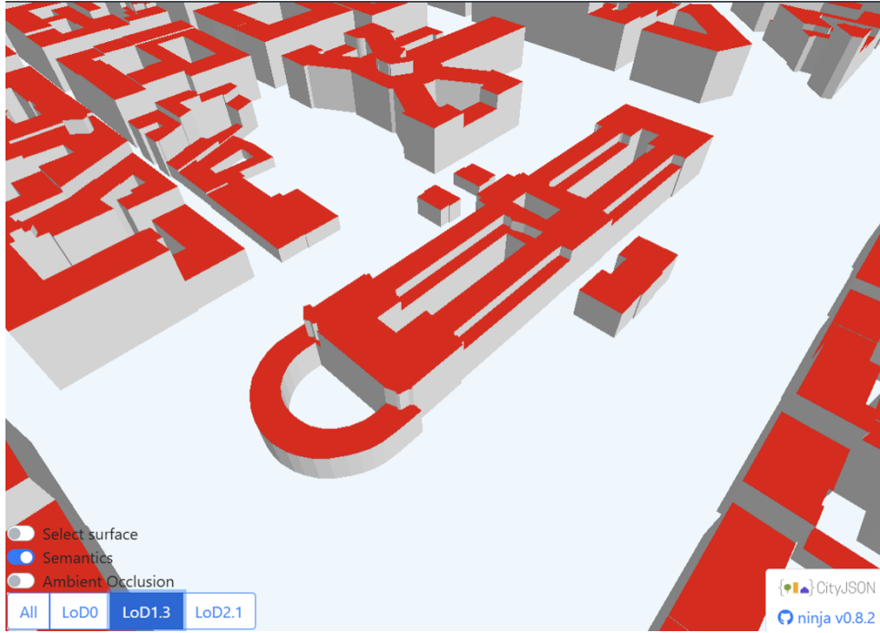
Figure 4.6: The same building at LOD1.3: a flat top, with no slope or roof-face information.
