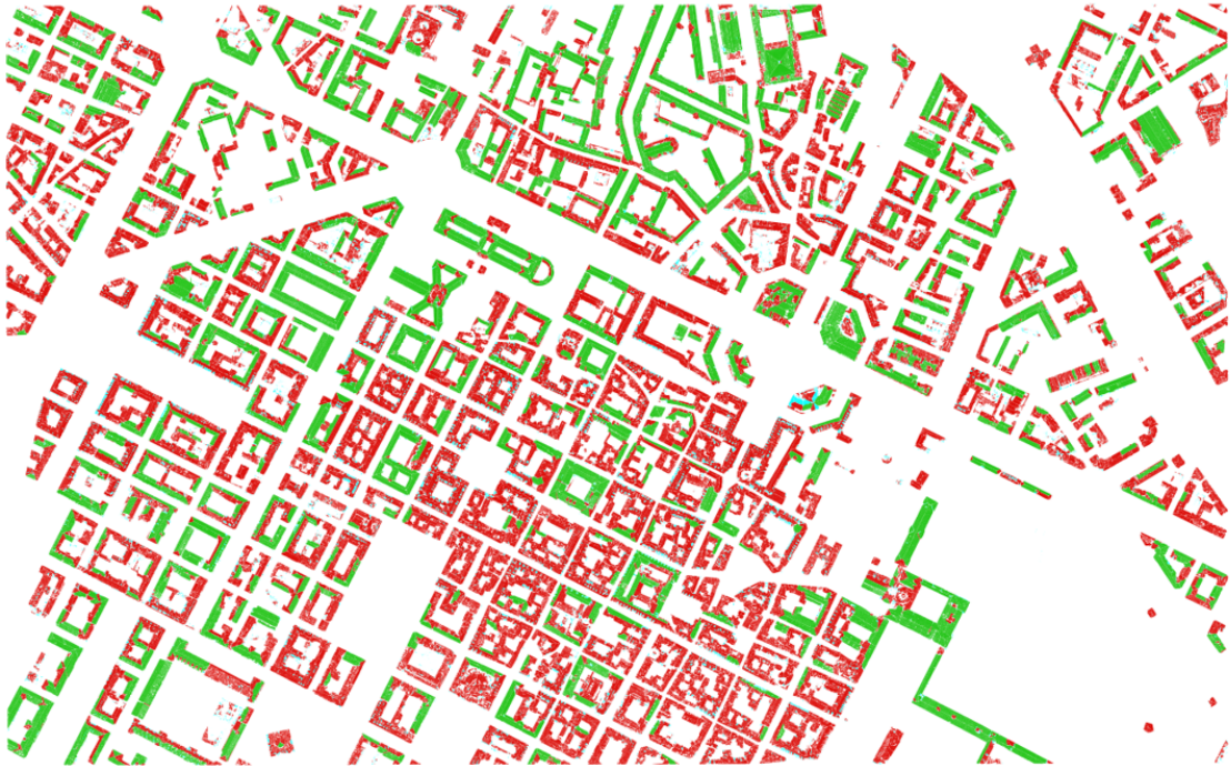
Figure 5.3: The classifier applied to the whole study area. Green = good roof (class 1), red = bad surface (class 2), cyan = window or obstruction (class 3). Obstructions are many in number but small in area, so at this scale they appear as scattered dots rather than large patches.
