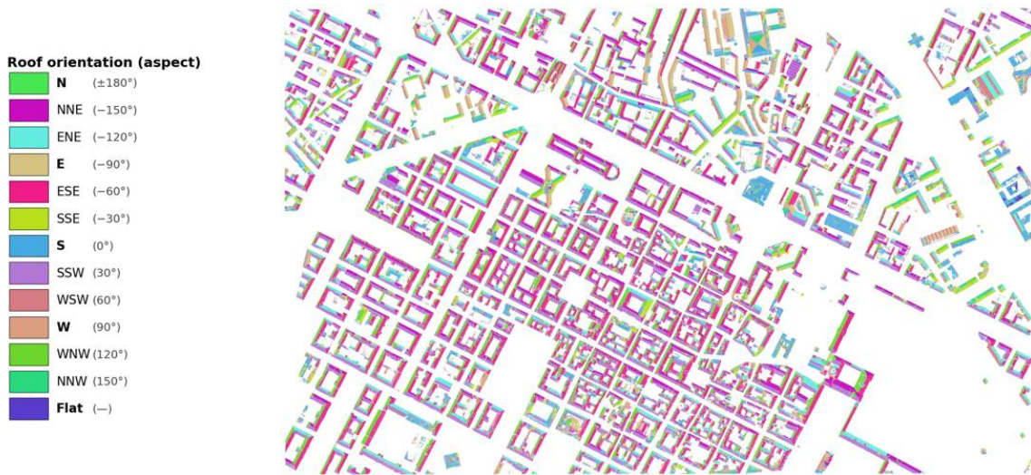
Figure 5.2: The vectorised roof segments over the study area, coloured by orientation class: a flat class for near-horizontal roofs, plus twelve 30^\circ sectors around the compass (here 0^\circ points south, -90^\circ east and 90^\circ west). The twelve sectors cover the four cardinal directions and two intermediate directions within each quadrant, so each colour is one of the twelve orientation classes. This is the segmentation result that the following steps work on.
