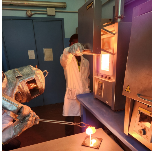
Figure 2.1: Molten GC2 glass being poured on a metal plate at the end of the casting process
