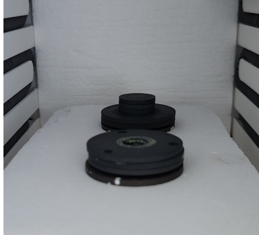
Figure 2.16: Samples placed inside of Carbolite 1300 furnace with weights placed on top before thermal treatment process was initiated.
