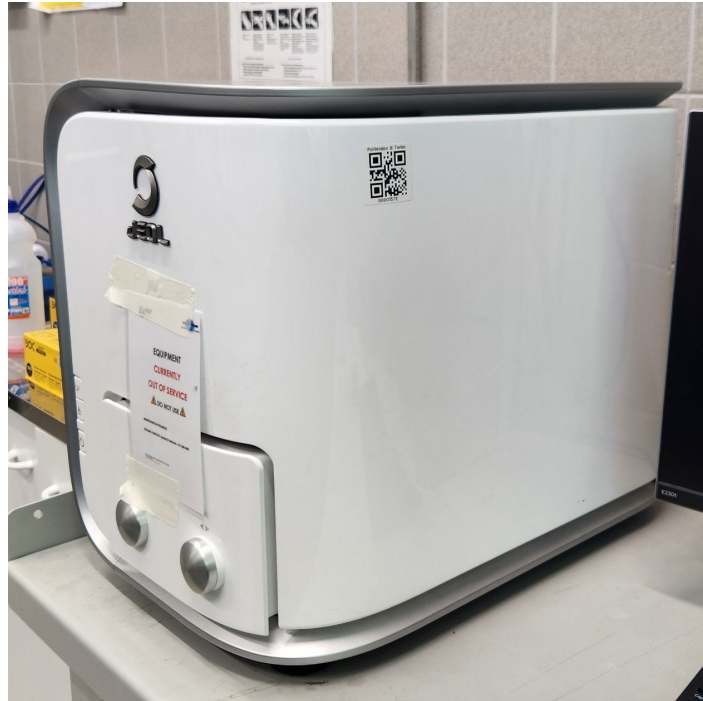
Figure 2.23: SEM JEOL JCM-6000Plus
