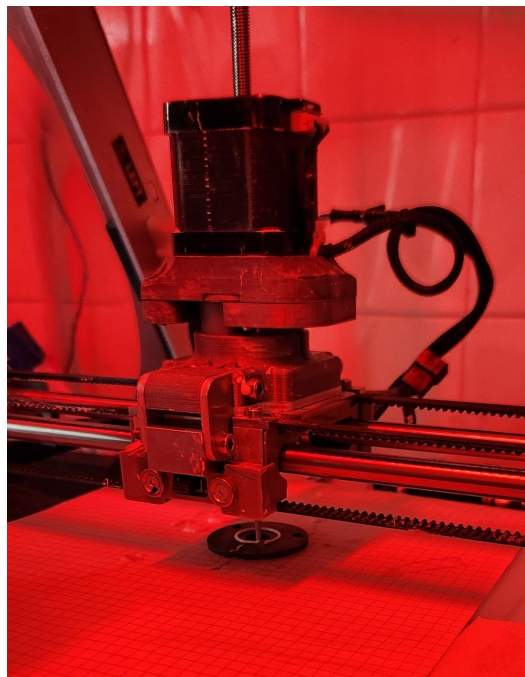
Figure 2.11: Robocasting process in progress.
