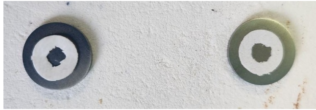
Figure 2.14: Metal samples with tape placed on them before joining process.
