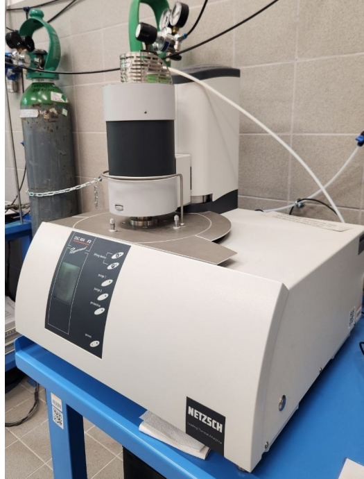
Figure 2.6: DSC 404 F3 Pegasus by Netzsch.
