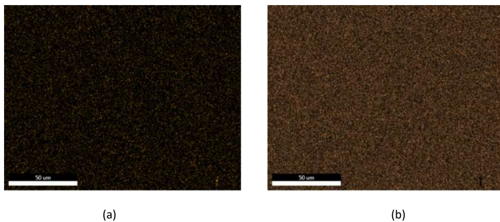
Figure 4.1.9: EDS elemental maps of the gold-sputtered Ni 725 gauge surface prior to tensile testing.(a) Ni map (b) Au map.
