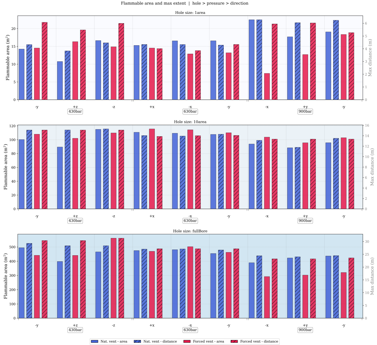
Figure 3.12: Summary of the cloud projection of the flammable area and maximum reach at steady state for all the cases organised by a hierarchy of hole size, then pressure, then direction.
