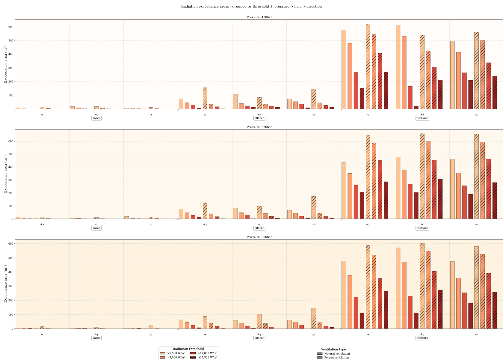
Figure A.36: Summary of the radiation scores at steady state for all the cases organised by a hierarchy of pressure, then hole size, then direction.
