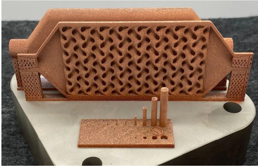
Figure 9: CuCrZr gyroid sample [29]
