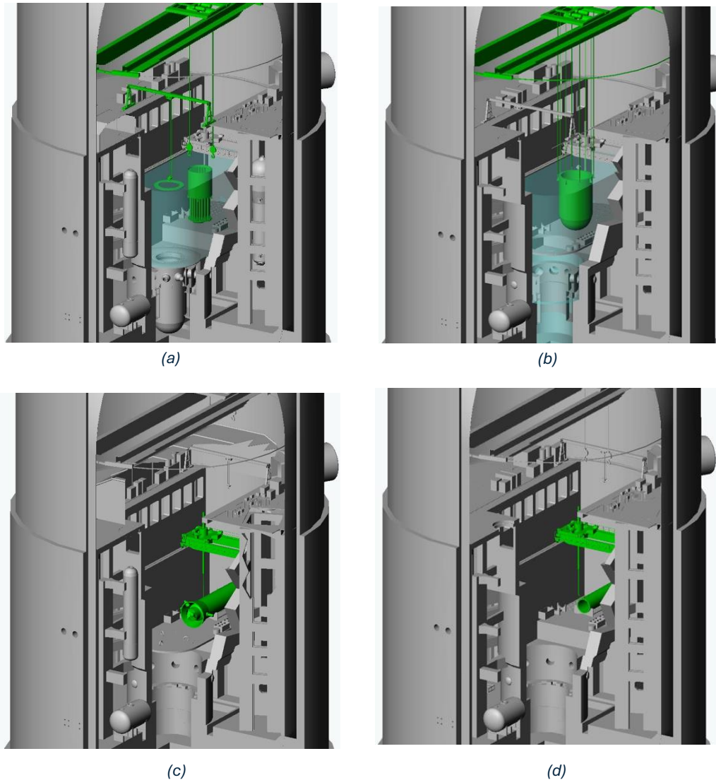
Figure 7.1 (a) internals removal, (b) vessel removal, (c) SG cutting, (d) pressurizer cutting
