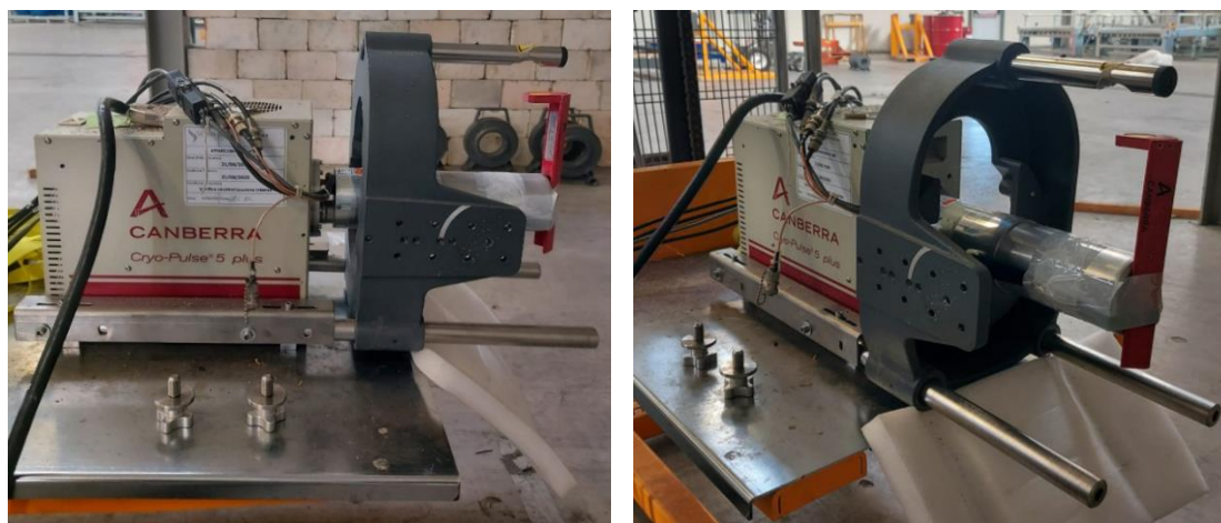
Figure 5.2 ISOCS system during calibration with reference source positioned in front of the detector
