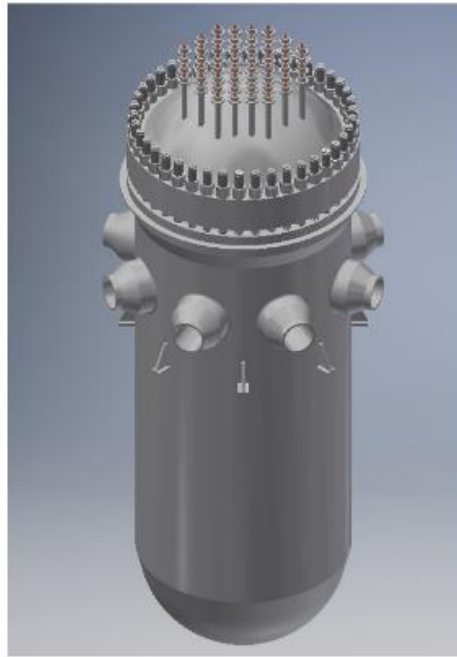
Figure 3.2 General view of the RPV
