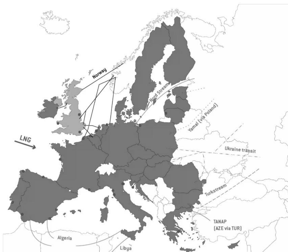
Figure 2.1 - Major natural gas import routes and LNG entry points in Europe before the post-2022 supply reconfiguration
