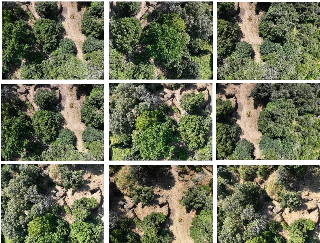
Figure 56. Sample UAV images acquired during the photogrammetric survey showing the overlap required for SfM processing.
