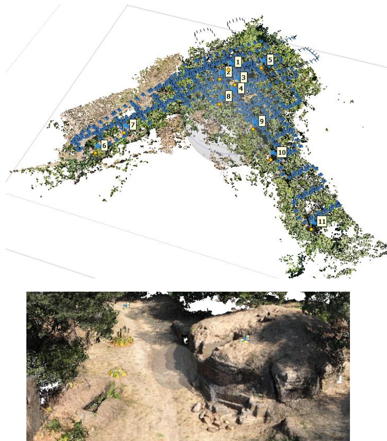
Figure 57. Dense point cloud generated in Metashap through Structure-from-Motion processing of UAV imagery acquired within the Via degli Inferi study area.
