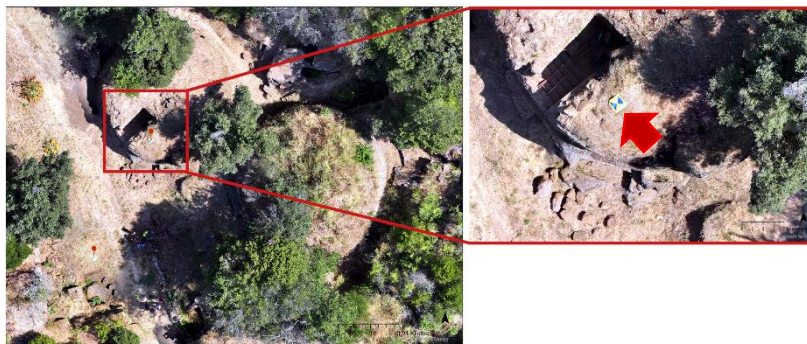
Figure 53. Example of Ground Control Point (GCP) placement used for UAV georeferencing within the Via degli Inferi study area.
