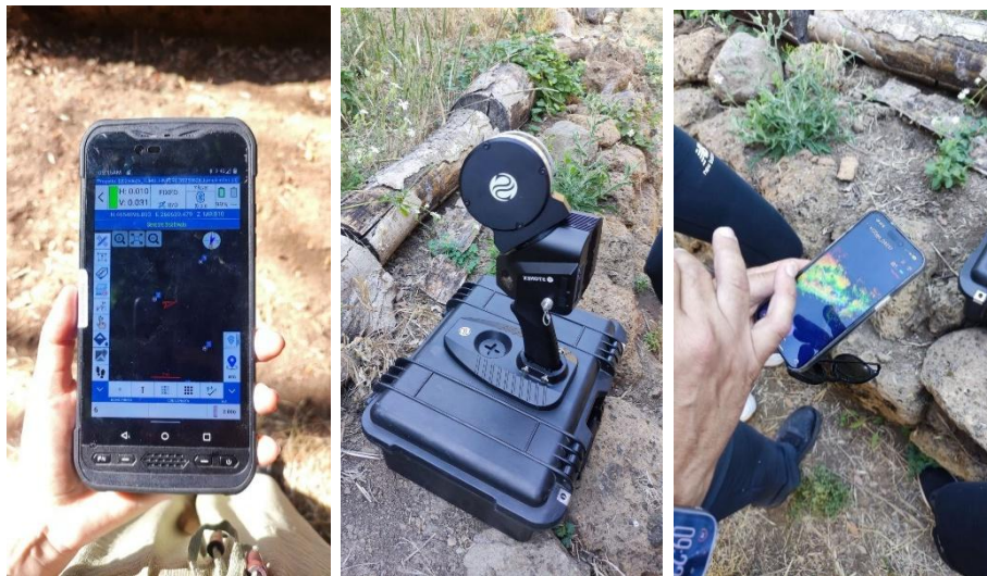
Figure 60. Mobile LiDAR SLAM Survey process documentation
