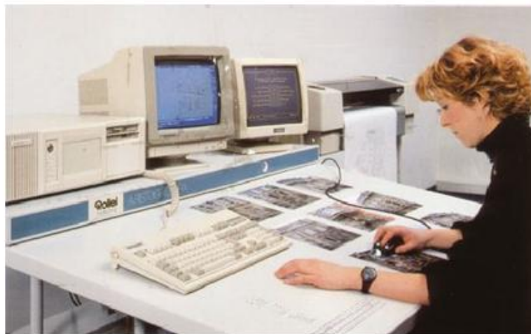
Figure 42: Rollei MR2 multi-image restitution system (ca. 1990)
