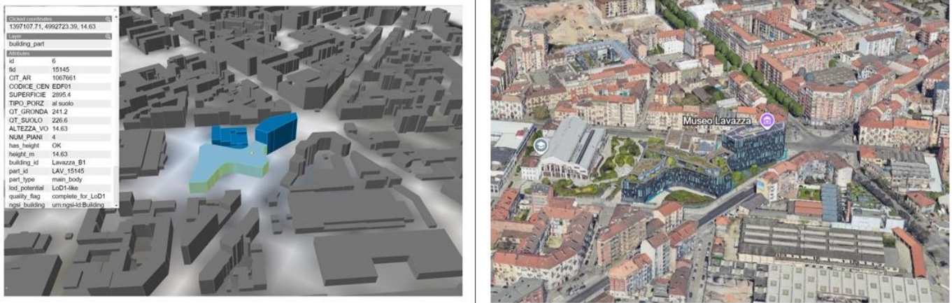
FIGURE 4.4 INTERACTIVE CLICKABLE 3D MODEL EXPORTED WITH QGIS2THREEJS, SHOWING COMPONENT ATTRIBUTES AND NGSI-LD-STYLE IDENTIFIERS. SOURCE: AUTHOR'S ELABORATION.
