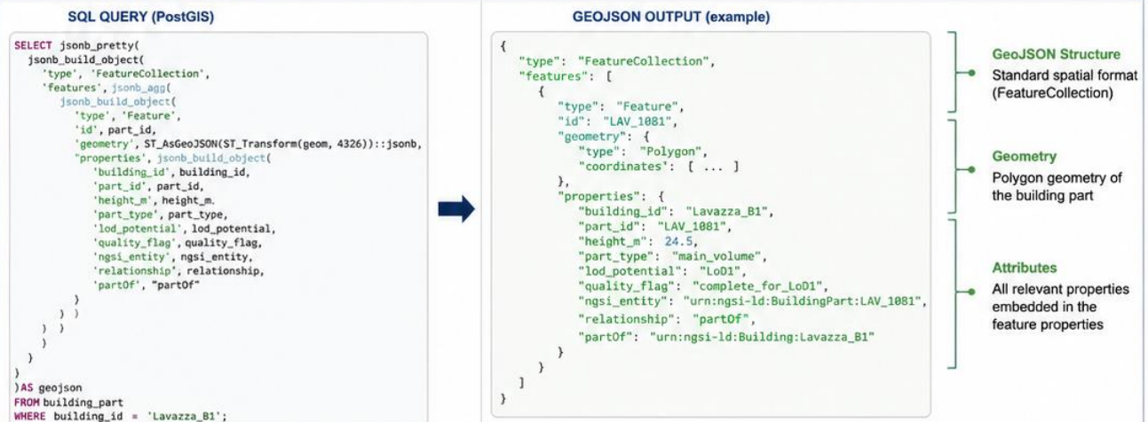
FIGURE 4.3 EXAMPLE OF GeoJSON OR NGSI-LD-STYLE JSON OUTPUT GENERATED FROM POSTGIS. SOURCE: AUTHOR'S ELABORATION.
