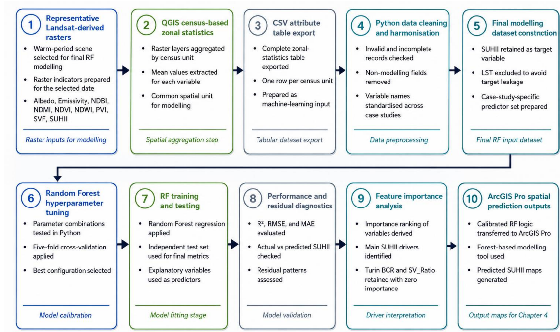
Figure 4.1. Workflow for warm-season SUHII modeling using Random Forest regression, from data preparation and hyperparameter tuning to validation, feature-importance analysis, and spatial prediction.
