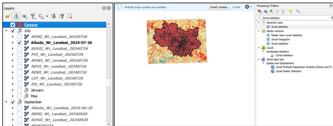
Figure 3.9. QGIS workspace used to organize the Landsat-derived raster layers and the census-section polygon layer before zonal aggregation.
