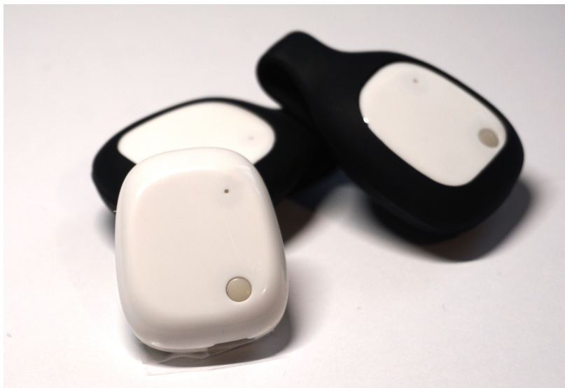
Figure 4.2: MetaWear wearable device used for live IMU acquisition and validation.
