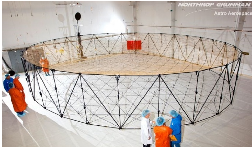
Figure 3.8: Typical cable-supported reflector architecture based on the AstroMesh concept. A deployable perimeter structure supports a pretensioned cable network that maintains the reflective surface geometry. @Credits from [7].
