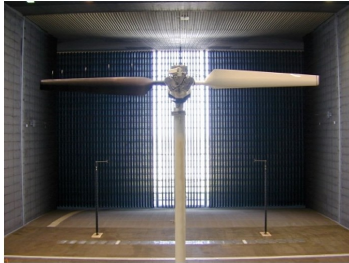
Figure 7.24: View of the full-scale wind-turbine model tested in the NASA Ames wind tunnel [11].
