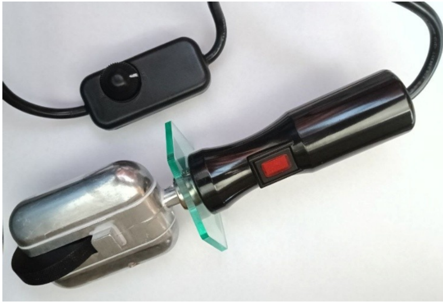
Figure 3.7: Manual thermal sealer used for balloon's production. It is provided with a temperature regulator.
