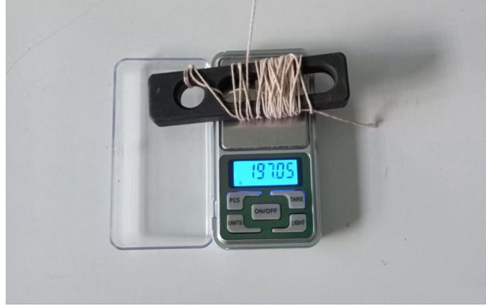
Figure 3.12: weighting of second balloon after retention test
