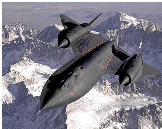
Figure 3.10: Chined fuselage of an SR-71 Blackbird.
