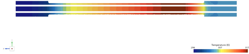
Figure 4.19: Temperature distribution on the stainless steel multi-channelled test object for a certain Reynolds number, as reconstructed by STAR-CCM.
