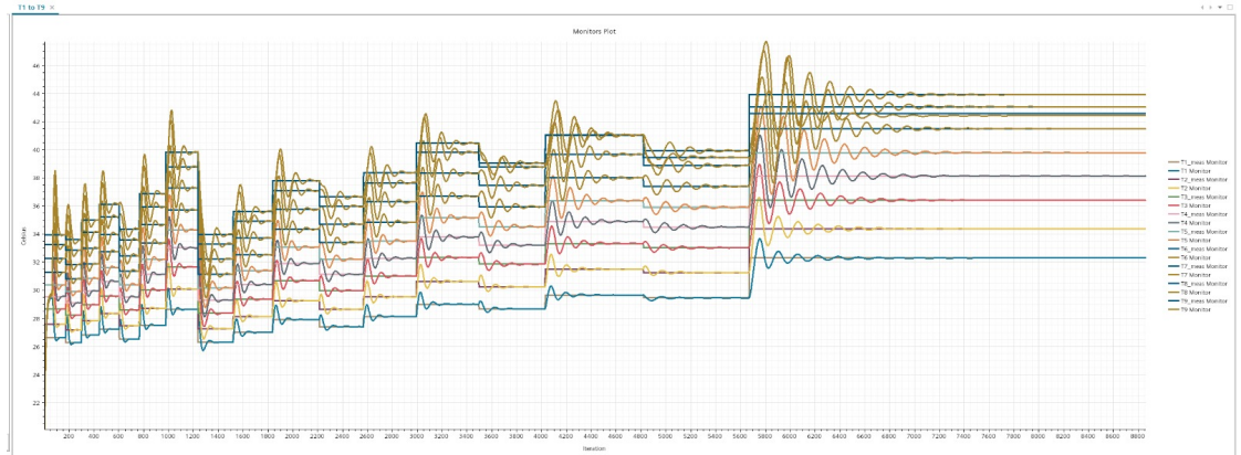
Figure 4.20: STAR-CCM monitor plot for the model and experimental temperatures over solver iterations.
