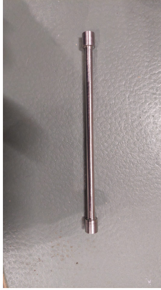
Figure 4.7: Example of a machined test object. In this case (Inconel 939), the machined portion is longer, as it also includes the length of the copper bar.
