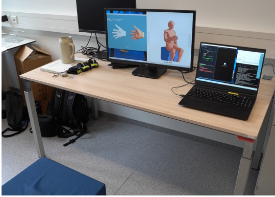
Figure 2.9. Laboratory setup: the subject was seated on the cube stool, with the laptop (on the right) showing the UI interface to control the experiment and plot the real-time EMG signal, and the supplementary monitor (left) which showed the Position Interface on the right side and the Virtual Hand Interface on the left side. On the desk, different sizes of the EMG-bracelets, and the reference electrode.
