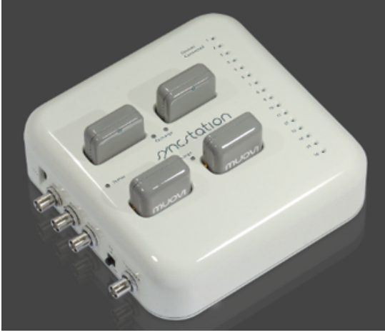
Figure 2.1. Sync-station containing four Muovi probes (in gray).
