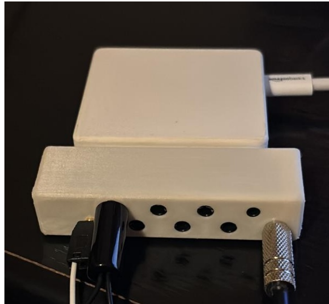
Figure 2.1: MotemaSens amplifier used for ECG and EDA signal acquisition, shown with the acquisition cables connected.
