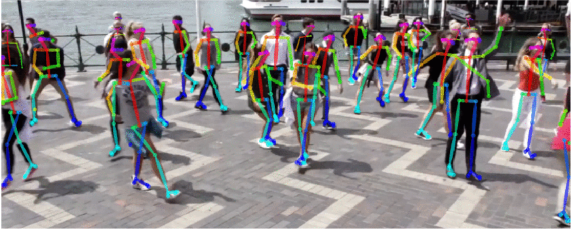
Figure 2.8: Typical output of OpenPose for multi-person 2D pose estimation. Adapted from [16].
