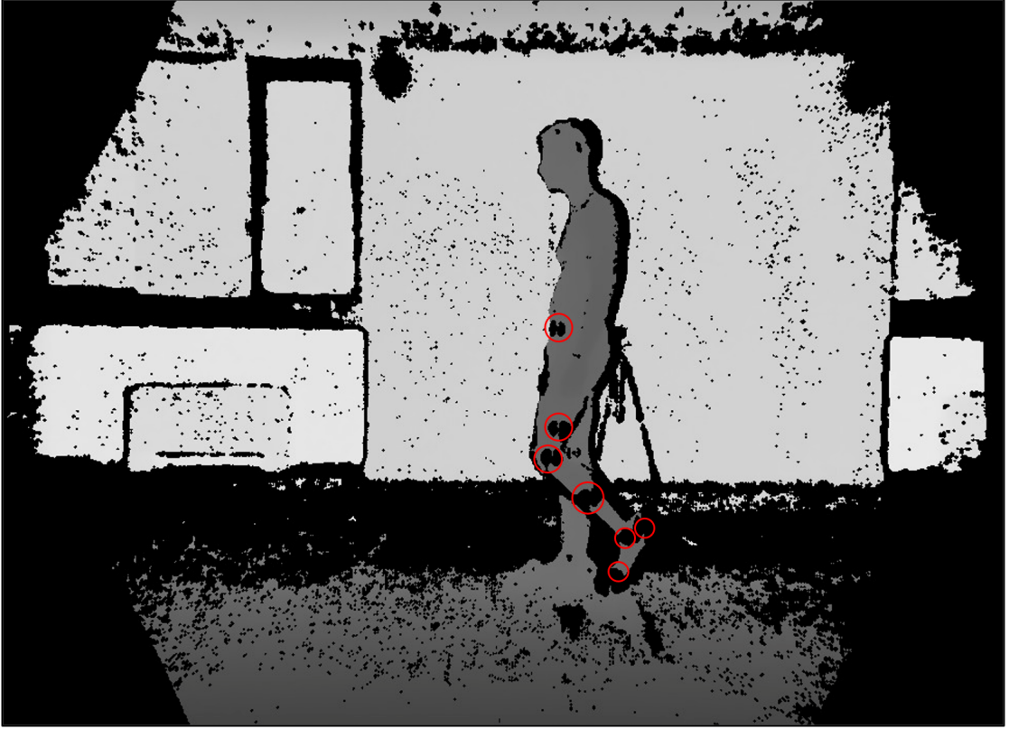
Figure 5.1: Example of depth artifacts observed during the simultaneous ML and MB acquisition. Black pixels are visible in correspondence with reflective markers on the foreground leg and foot, reducing the available depth information.
