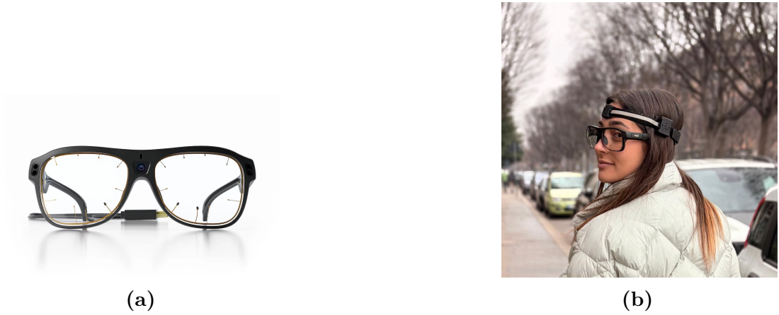
Figure 3.4: Tobii Pro Glasses 3 used in the present study: device (a) and wearing configuration during data acquisition (b).
