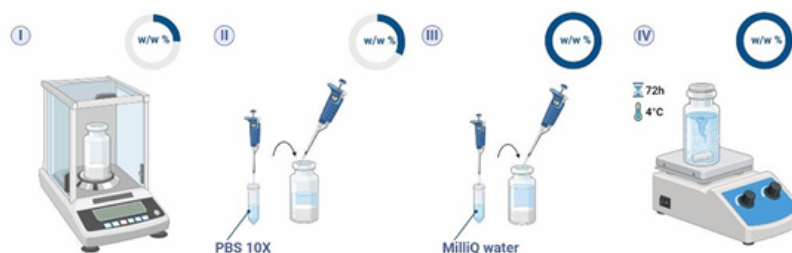
Figure 3.1: Schematic representation of the hydrogel preparation steps. I: weighing poloxamers; II: addition of 10X PBS; III: addition of MilliQ water; IV: stirring at 4°C for 72 hours. Created by Biorender
