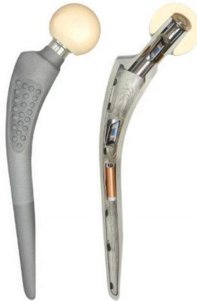
Figure 21: Hip implant instrumented with eight temperature sensors along the neck and shaft and four strain gauges to monitor multi-axis forces at the prosthetic head and stem.
