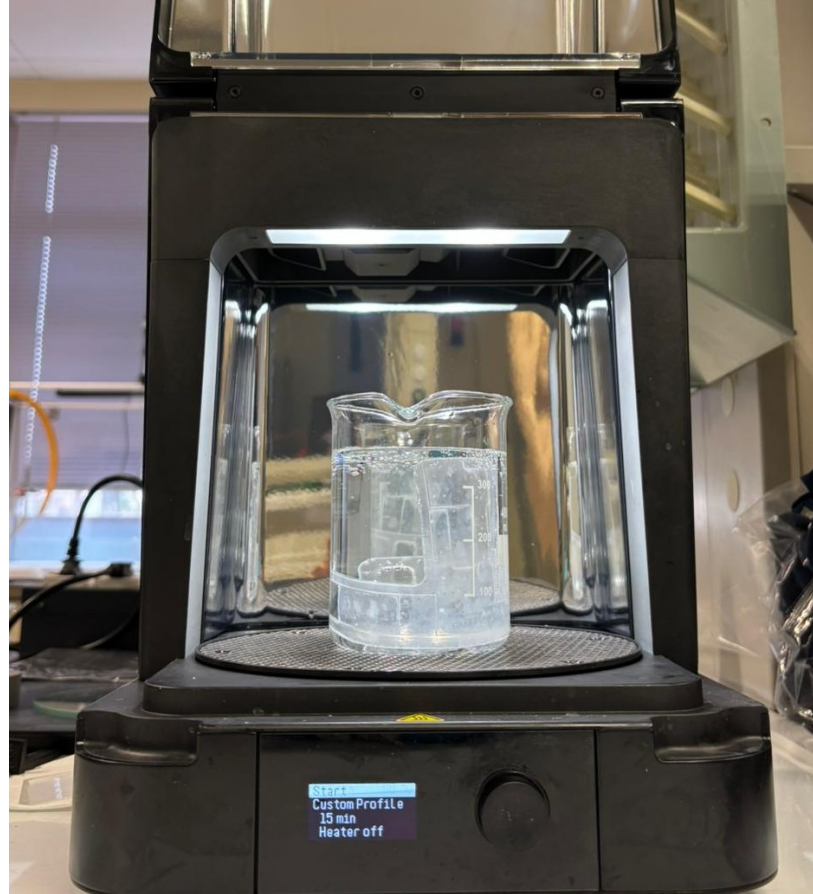
Figure 3.24: Resin case undergoing post-curing process in Form Cure V1 unit. Protocol conducted in the Advanced Biointerfaces Technologies Laboratory, IIT-CBN.
