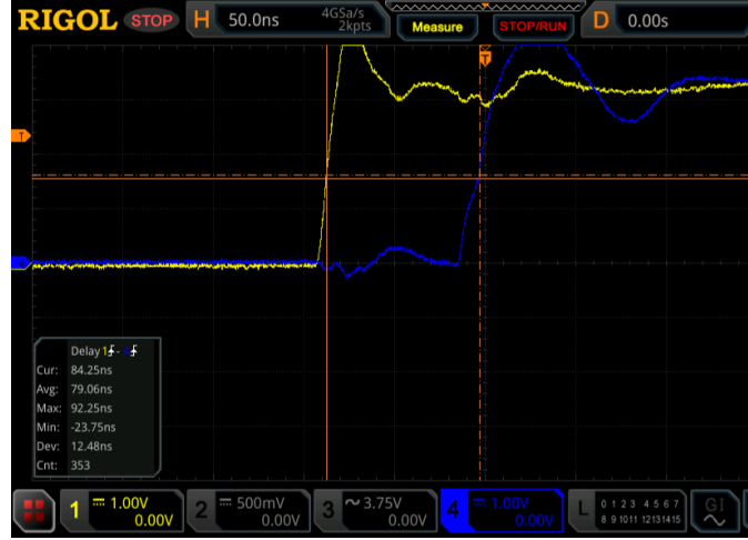
Figure 6.4. Oscilloscope measurement of the FPGA-internal latency ( \tau_{\text{FPGA}} ) . CH1 (yellow) probes the comparator signal entering the FPGA input pin; CH4 (blue) probes the corresponding GPIO edge on the sticky_mask output. The bottom-left panel reports the Delay 1→4 statistics accumulated over the acquisition (Cur, Avg, Max, Dev, Cnt), from which the per-session mean and standard deviation reported in Table 8.9 are extracted.
