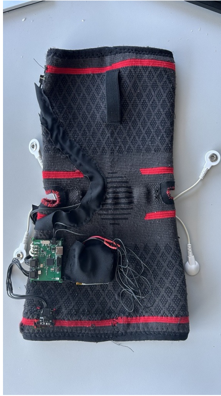
Figure 2.3: BioZ Knee Sleeve used to estimate knee flexion–extension movement and bioimpedance.
