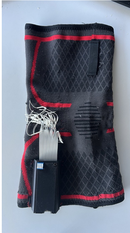
Figure 2.2: Temperature Knee Sleeve used for spatial temperature monitoring around the knee.
