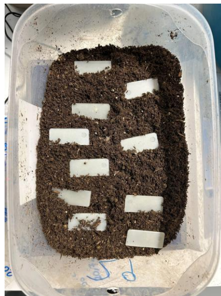
Fig 91. The placement of 1mm samples inside the composting reactor
