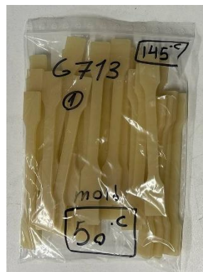
Fig 10. A sample of a dumbbell-shaped specimen, which was moulded at 50°C
