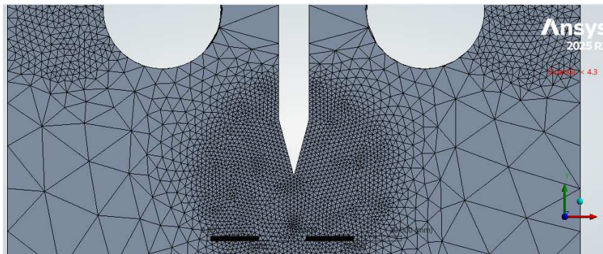
Figure 4.7: meshing of the crack tip and pin-hole
