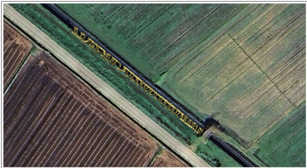
Figure 3.4 – Aerial section of the mapped field derived directly from the QGIS worksheet, in which the bathymetric data are processed, which shows the spatial trajectory of the acoustic profiler during the bathymetric survey along the Cavo Lucca. The yellow dots represented in the figure represent the points of the grid where the profiler effectively performed measurement, defining the scanning grid that guarantees a complete and high-resolution three-dimensional mapping of both the morphology of the bottom of the canal and of the internal velocity field.
